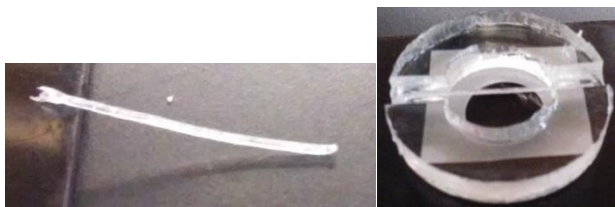
Figure 17: Dehydrated Pluronic cylinder a) resting against acetate slide to show stiffness and b) placed in PDMS mold.
