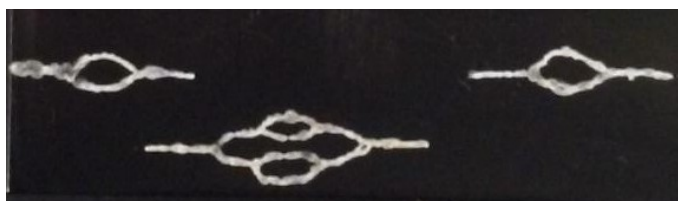
Figure 31: Pluronic bifurcations via hand-drawn extrusion
