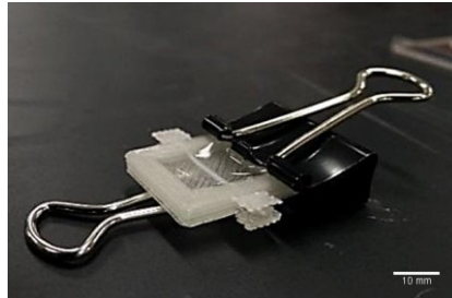
Figure 25: Two Piece Mold with PVA channel and fibrin scaffold forming
