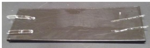
Figure 16: Multiple sizes of Pluronic cylinders extruded from 1 mL syringe (left) and 23G needle (right).
