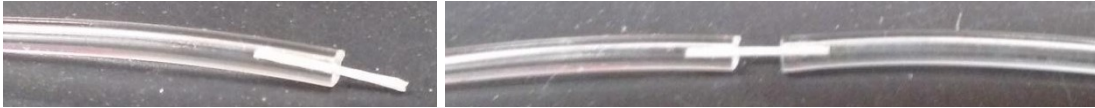
Figure 40: "Lateral tube-loading" loading mechanism: a) Sacrificial material is inserted into one tube and then b) the other tube is moved laterally into place over the other end of the cylinder.
