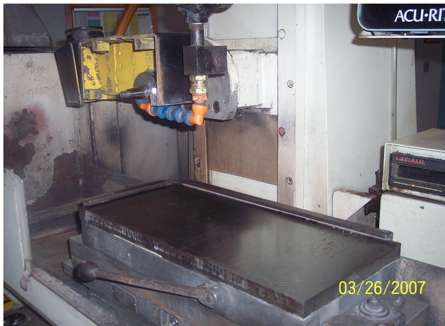
Figure 16: Surface Grinder Fixture
