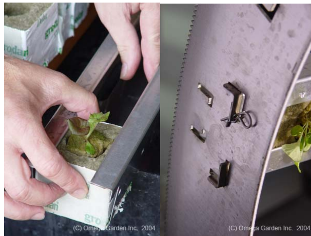
Figure 55 Omega Garden channel and adapting plate details (Omega Garden).
