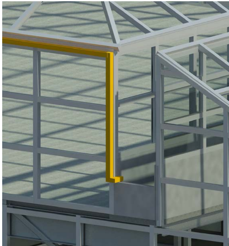
Figure 66 Gutter & Downspout Render.
