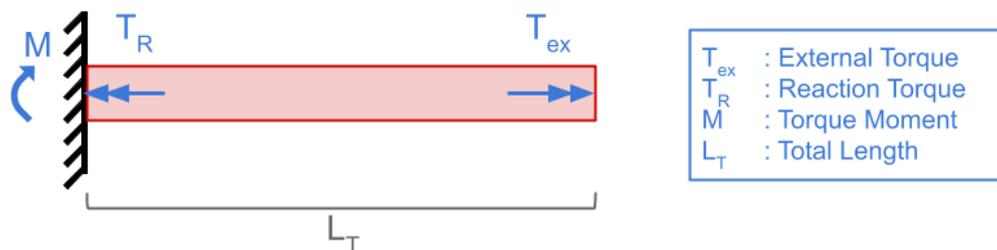
Figure 36: Torsion Along a Fixed Piling
