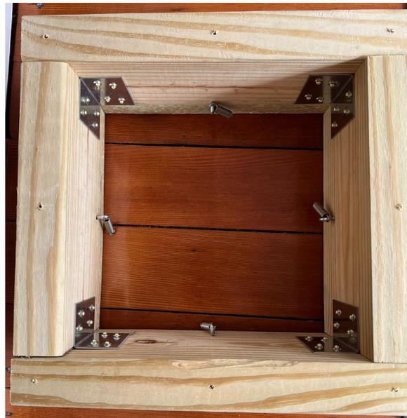
Figure 64: Square casing with corner brackets
