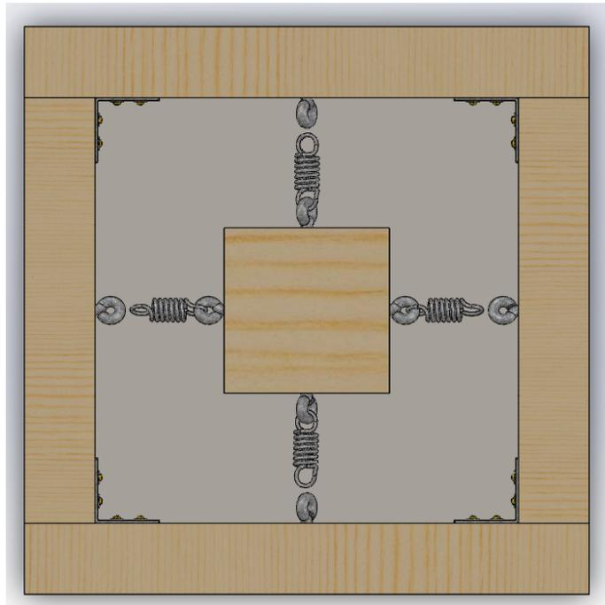
Figure 17: Bottom view of the proposed dock deformation mechanism assembly, outside of the 1 ft. x 1 ft. square enclosure is fixed to an existing fixed dock
