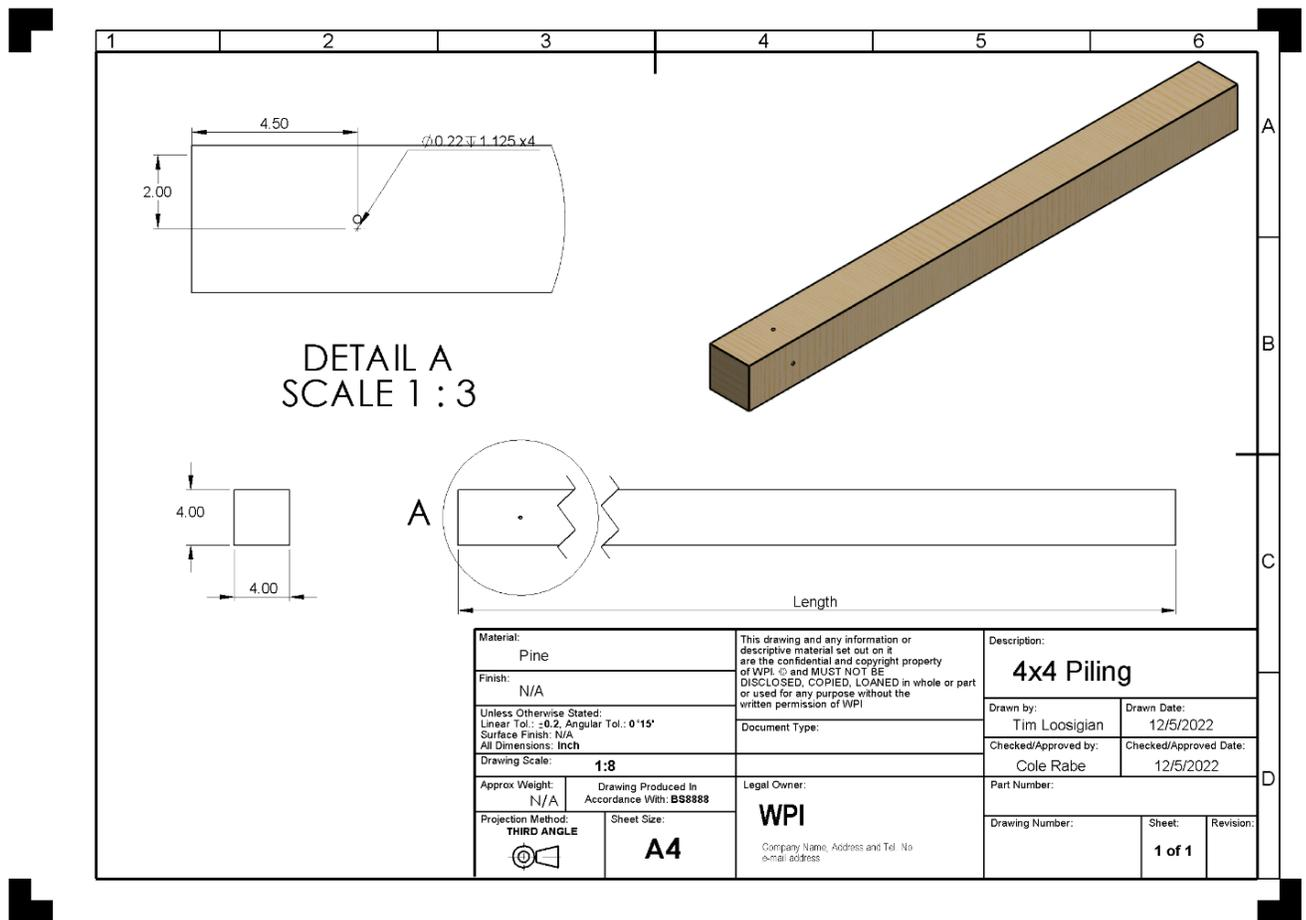
Figure 22: Technical drawing of the 3D modeled piling with predrilled holes
