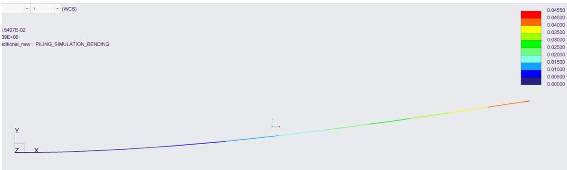
Figure 44: CREO Simulation for Traditional Bending Deflection (ft)
