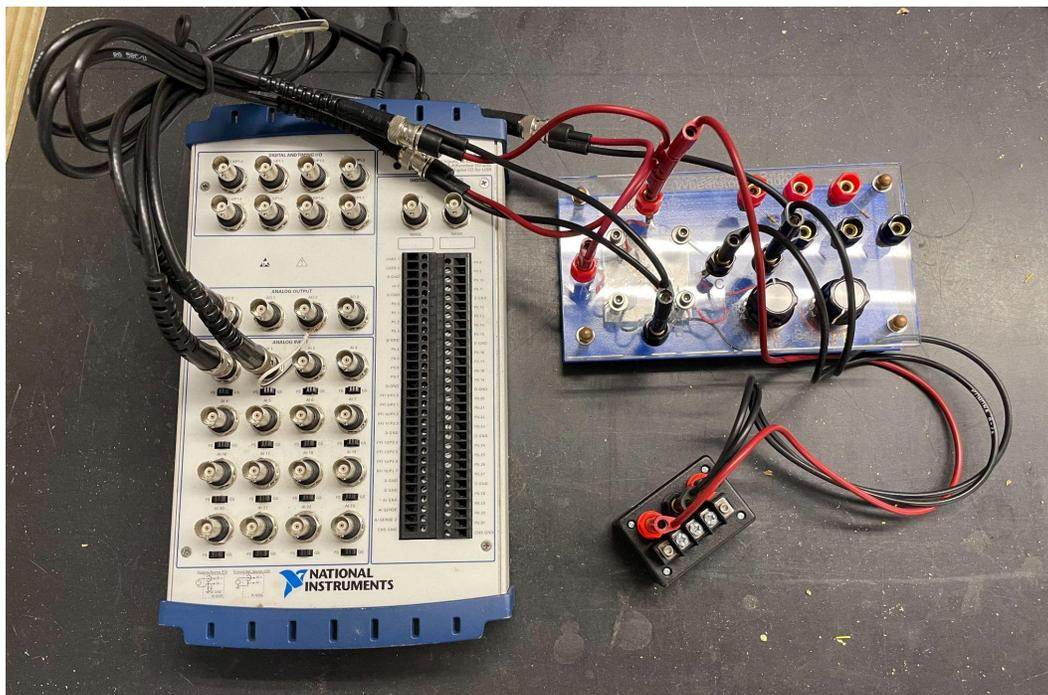
Figure 77: Wheatstone Bridge Set Up In Person
