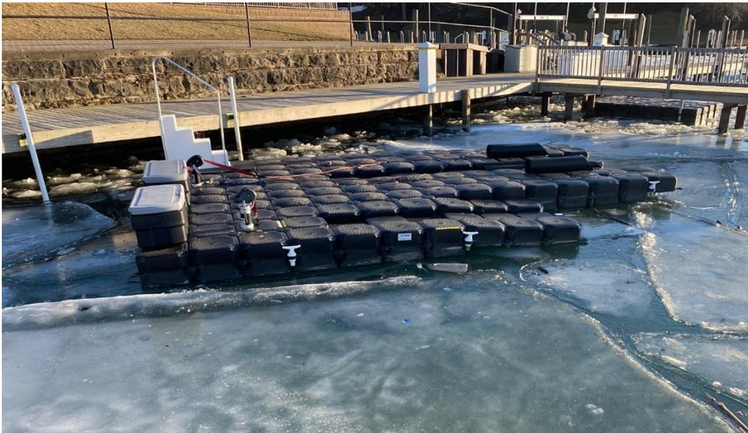
Figure 14: A Jet Dock surrounded with ice (*Winter Boat Dock | Discover Docks That Can Stay in Ice & Floating Cold Weather Boat Lifts for Winter - Jet Dock, n.d.*)
