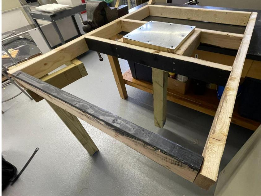
Figure 68: The frame constructed for testing with the mechanism inside
