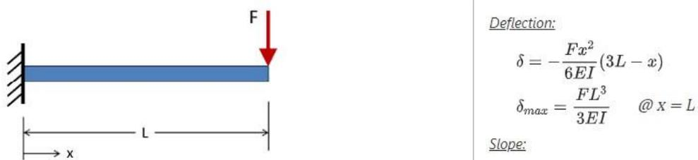
Figure 43: Diagram and Equation for Deformation Calculations (Beam Deflection Tables, n.d.)
