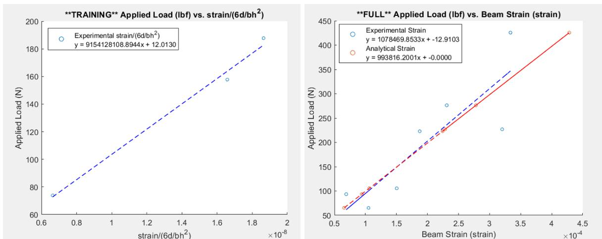
Figure 80a (left): Training data to calculate Young's Modulus of a 4x4 pressure-treated piece of wood
