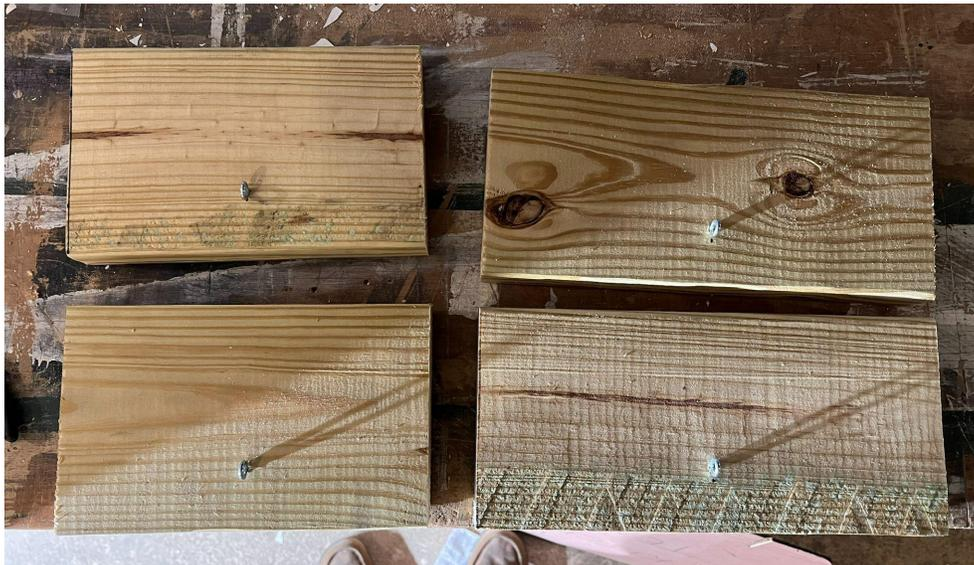
Figure 60: 9 in. and 12 in. square casing 2 in. x 6 in. wood pieces
