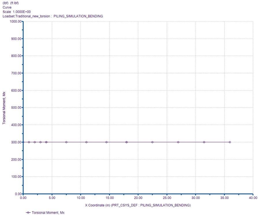
Figure 38: Torsional Moment Along Traditional Piling (lbf\*ft<sup>2</sup>)
