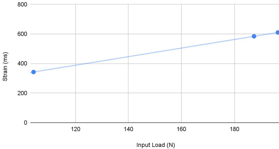
Figure 83: Applied load (N) vs. Strain (microstrain) graph for the fixed piling
