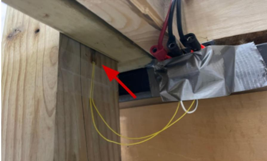
Figure 81: Traditional Fixed Piling Strain Gauge Location
