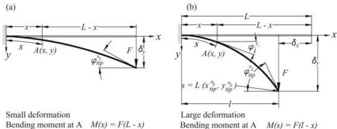
Figure 88: Comparing magnitude of bending moment and deflection angle (Saha & Ghuku, 2015)
