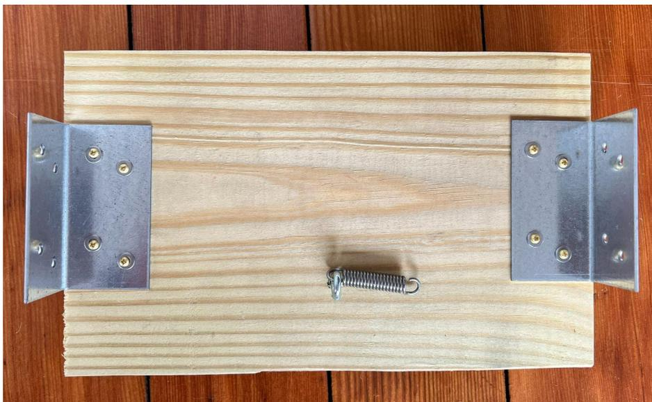
Figure 62: A wood piece with the addition of the corner brackets
