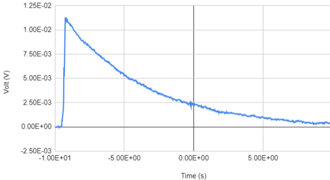
Figure 69: 1 lb weight being applied onto a Dytran 1051v4 Force Sensor
