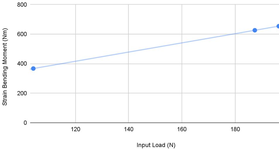
Figure 84: Applied load (N) vs. Bending Moment (Nm) graph for the fixed piling
