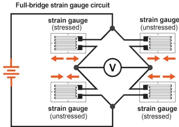
Figure 75: Full Wheatstone Bridge Diagram (Strain Gauges, n.d.)
