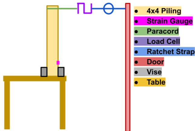
Figure 78: Experimental Setup Diagram
