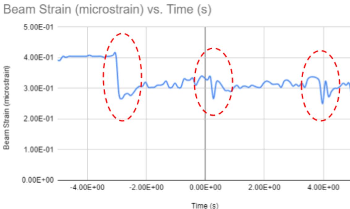
Figure 85: Beam Strain (microstrain) vs. Time (s) graph for the dynamic test on the fixed piling
