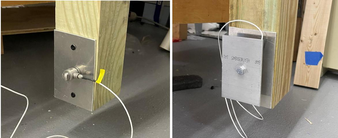
Figure 71a (left): Dytran Force Sensor Setup on Piling without top plate
