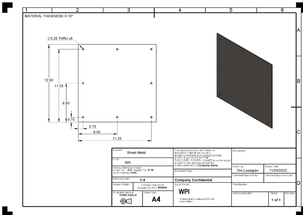
Figure 23: Technical Drawing of 12-in. x 12-in. Sheet Metal cover
