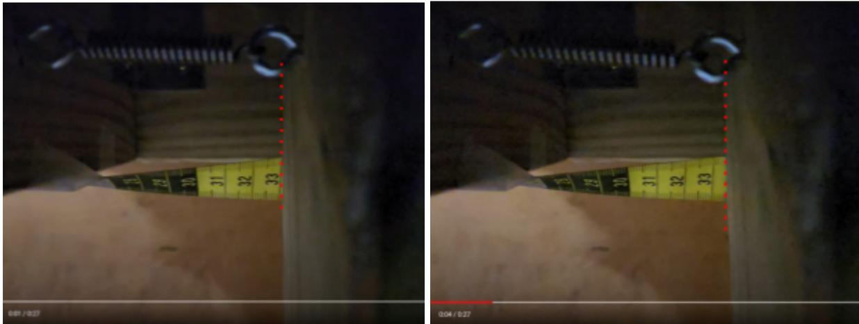
Figure 87a (left): Spring Displacement Before Impact (33cm)
