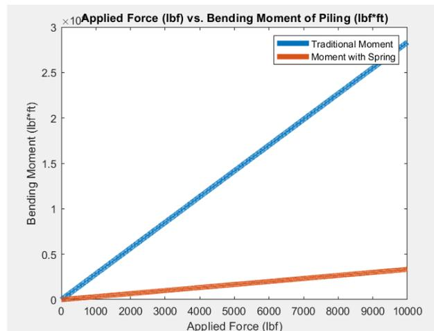
Figure 35: Applied Load (lbf) vs. Bending Moment of Piling (lbf\*ft)
