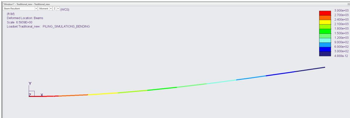
Figure 29: CREO Simulation of Traditional Fixed Piling (ft\*lbf)
