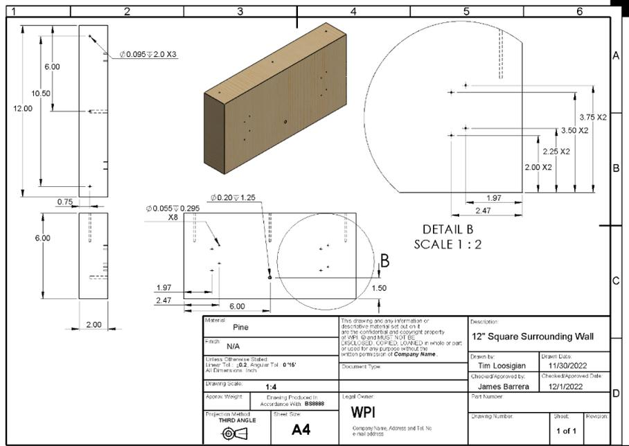
Figure 21: Technical drawing of 12-in. long 2-in. x 6-in. square surrounding wall with pre-drilled holes
