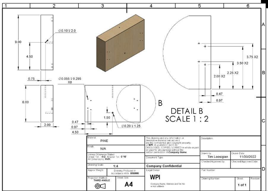
Figure 20: Technical drawing of 9-in. long 2-in. x 6-in. square surrounding wall with pre-drilled holes
