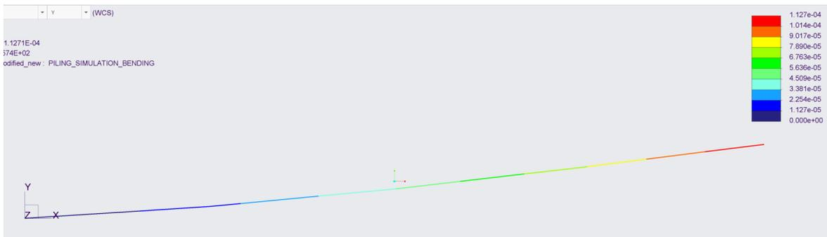
Figure 46: CREO Simulation for Modified Bending Deflection (ft)
