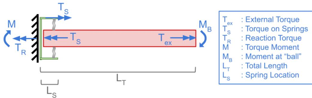
Figure 39: Torsion Along Modified Piling
