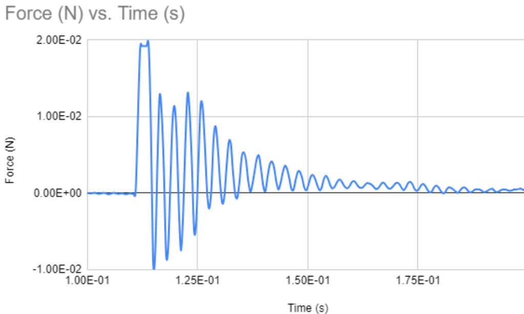
Figure 74: Force (N) vs. Time (s) of the spring mechanism with Dytran 1051v4 Force Sensor zoomed in
