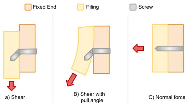
Figure 89: Comparing forces on the screws
