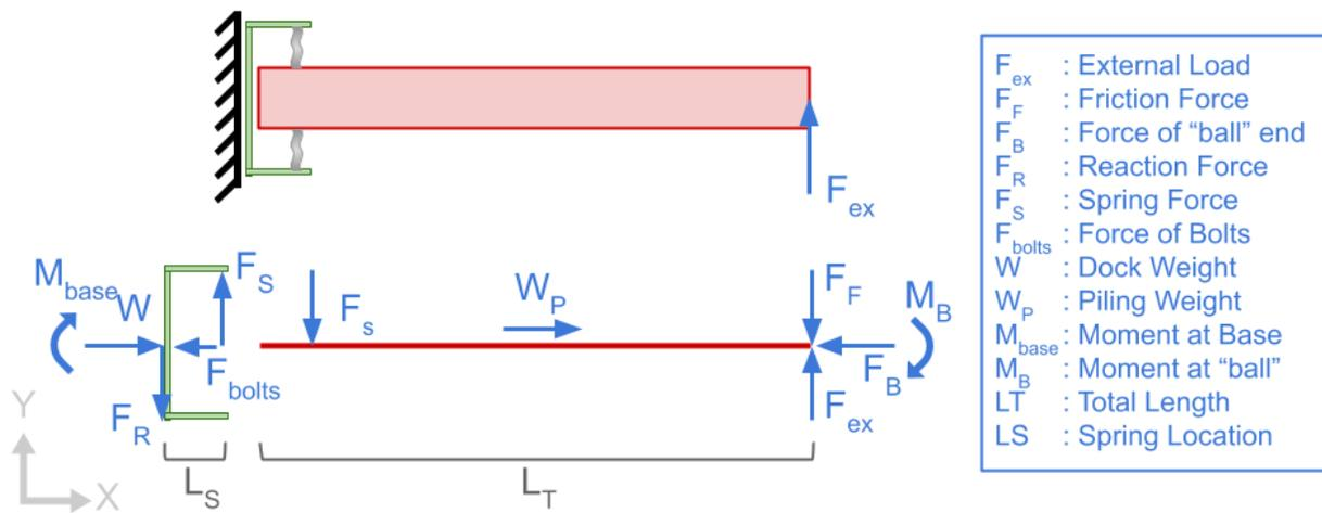
Figure 31: Modified Spring Piling FBDs
