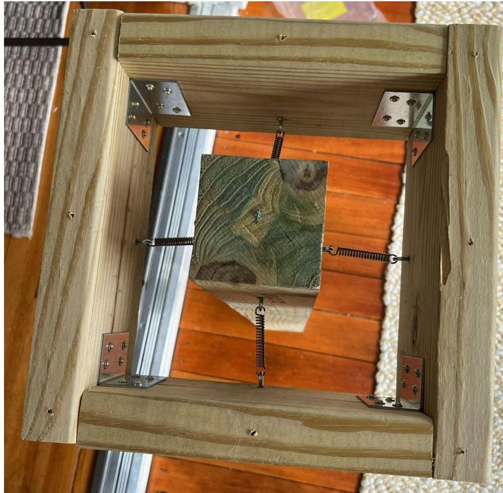
Figure 65: Square casing with the piling inserted
