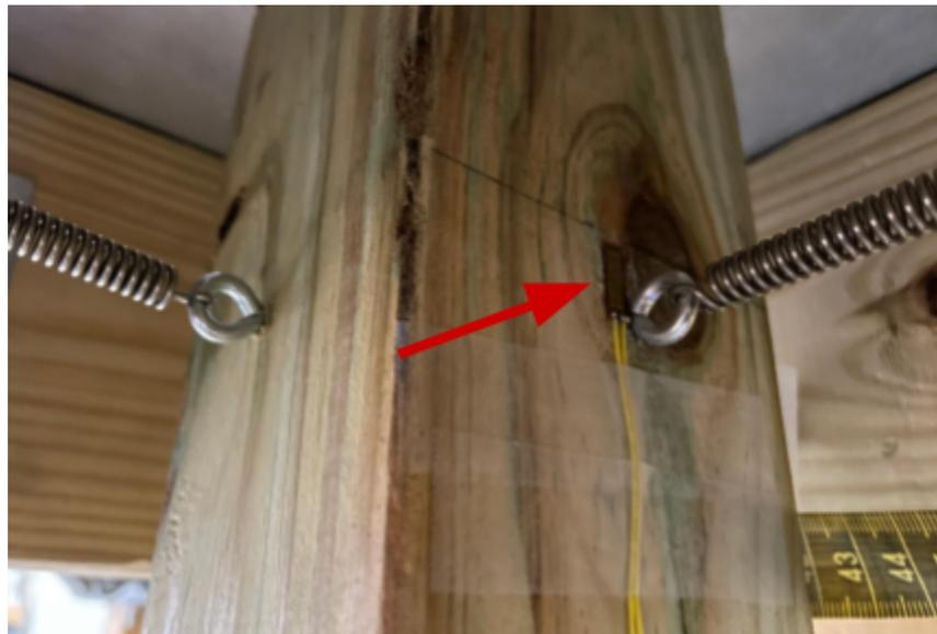
Figure 86: Modified Spring Piling Strain Gauge Location
