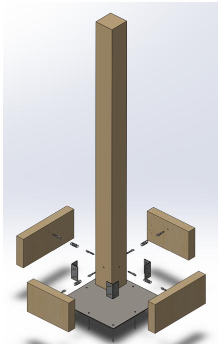
Figure 19: Exploded angled view of the proposed dock deformation mechanism assembly
