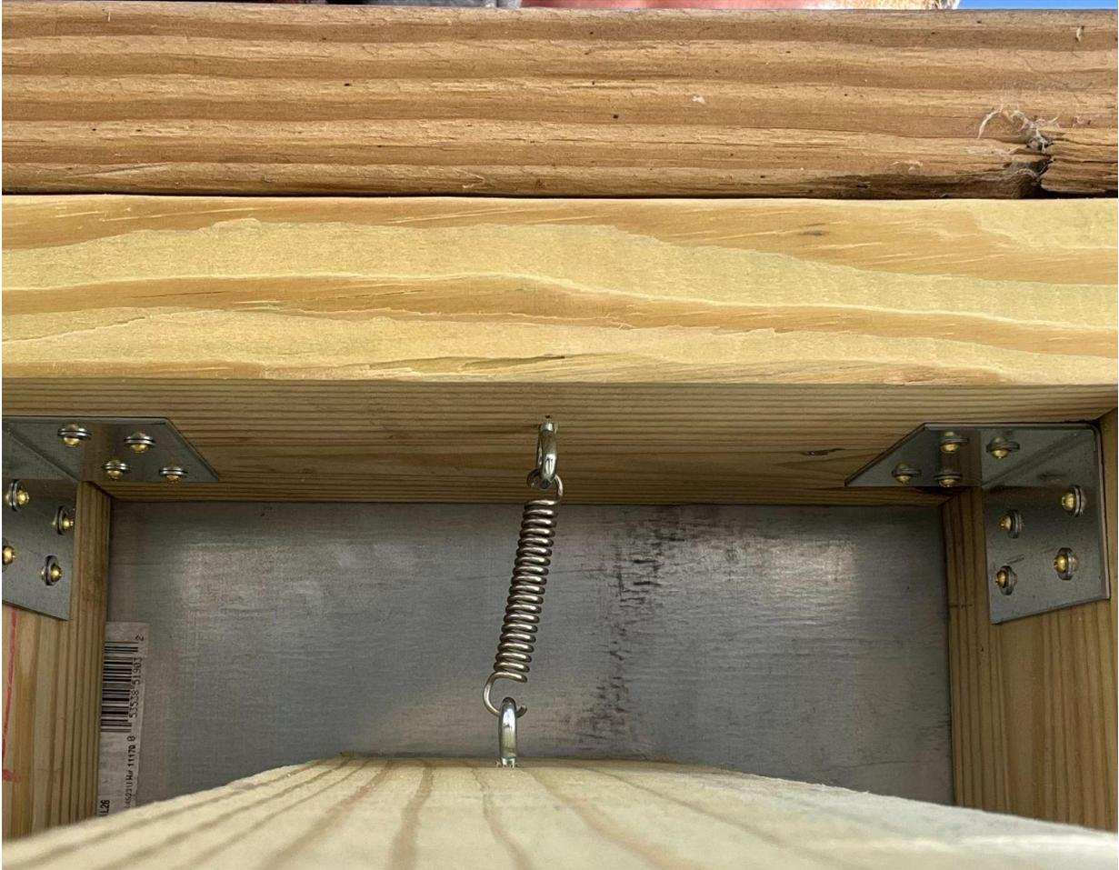
Figure 56: A stretched spring with horizontal movement on the initial prototype
