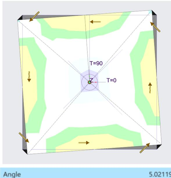
Figure 50: CREO Simulation for Traditional Twist (degrees)
