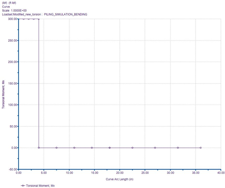
Figure 41: Torsional Moment Along Modified Piling(lbf\*ft<sup>2</sup>)
