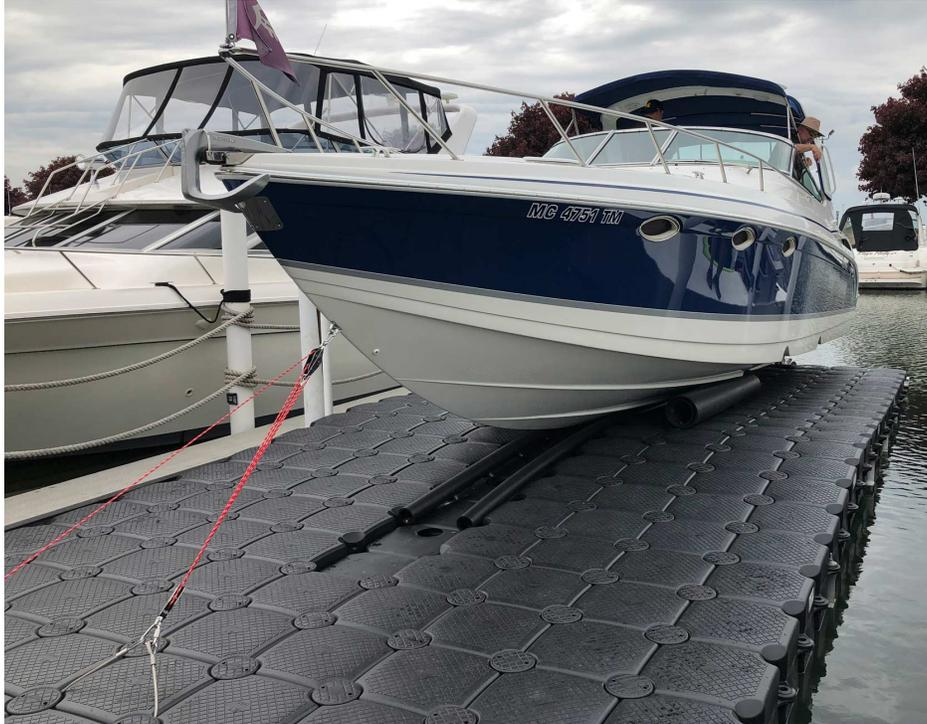
Figure 15: A Jet Dock supporting a large boat (*Great Lakes Jet Dock | Floating Boat Docks, Boat Lifts & Jet Ski Lifts – Jet Dock, n.d.*)
