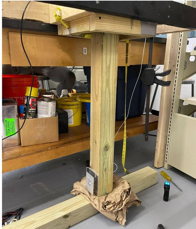
Figure 73: Dytran Force Sensor Setup for Spring Piling
