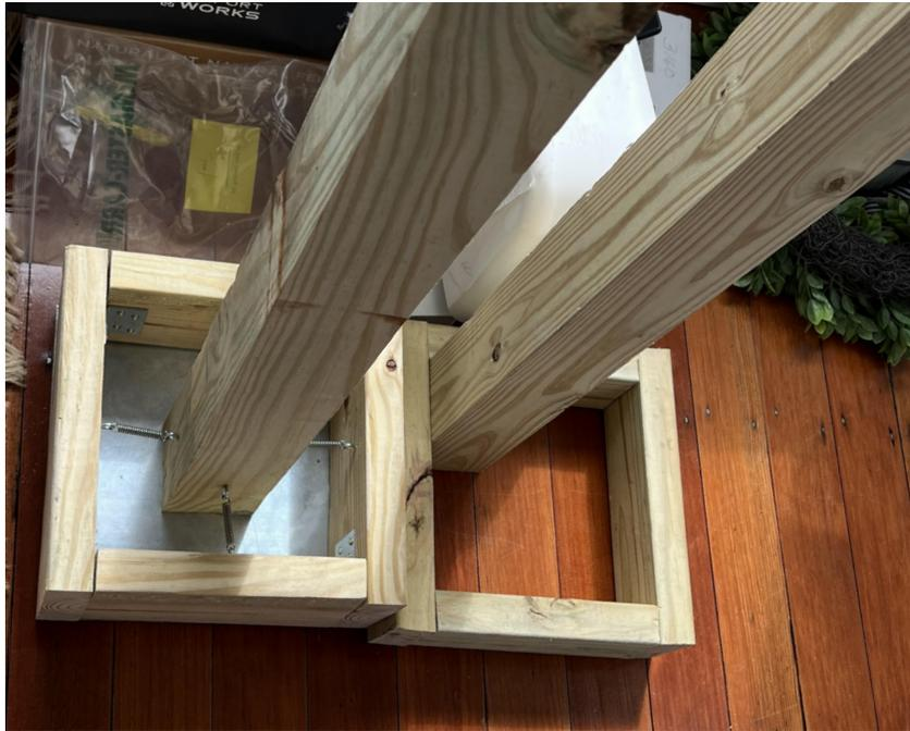
Figure 67: Final spring mechanism prototype (left) and the traditional fixed dock baseline testing representation (right)
