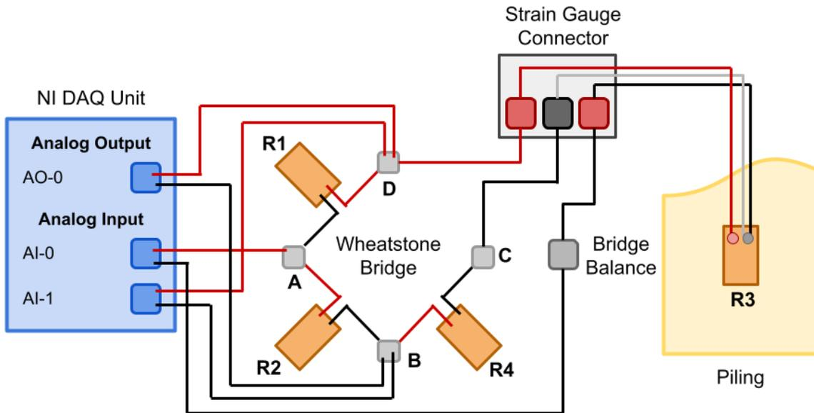
Figure 76: Wheatstone Bridge Set Up Diagram
