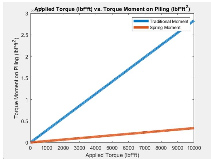
Figure 42: Applied Torque (lbf\*ft) vs. Torsional Moment on Piling (lbf\*ft²)
