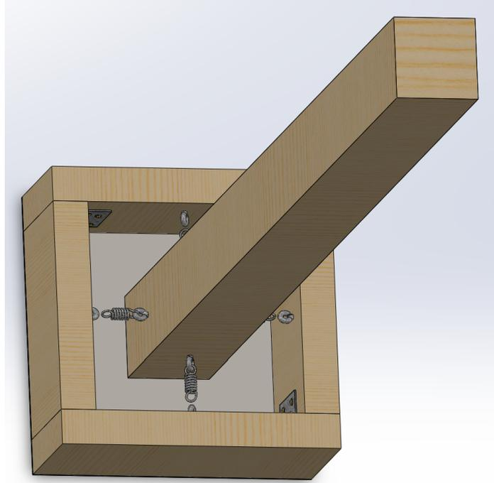
Figure 18: Angled view of the proposed dock deformation mechanism assembly
