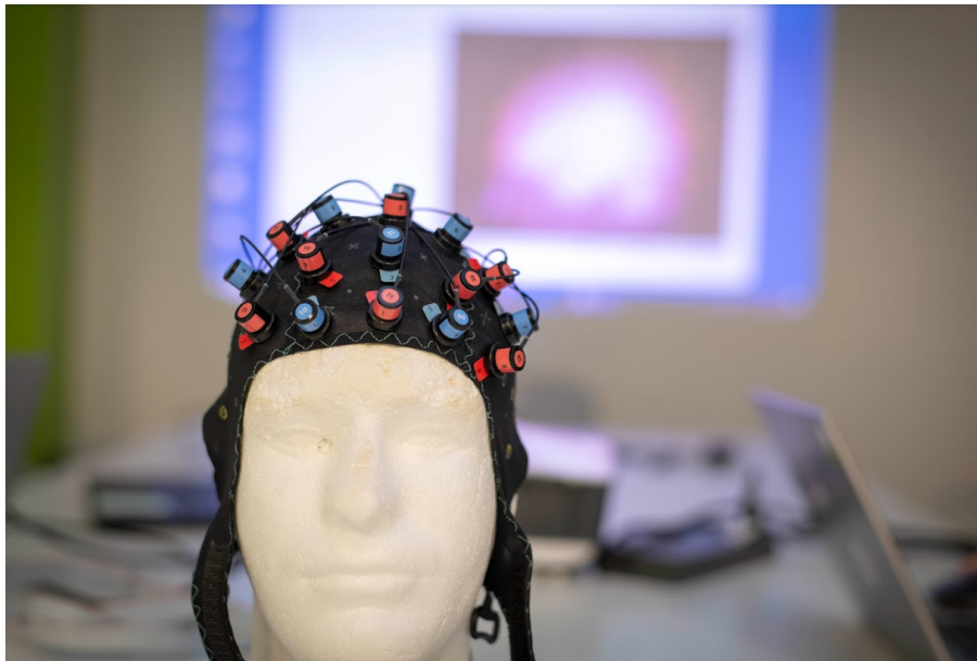
Figure 1: A picture of an fNIRS montage on an fNIRS cap. The montage is the series of red and blue optodes on top of the helmet/skullcap which is the fNIRS cap.
