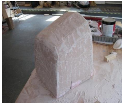
Figure 131: Nose Mold with Epoxy Stiffener
