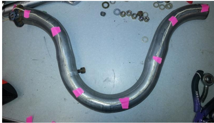
Figure 155: Exhaust Header Pipe
