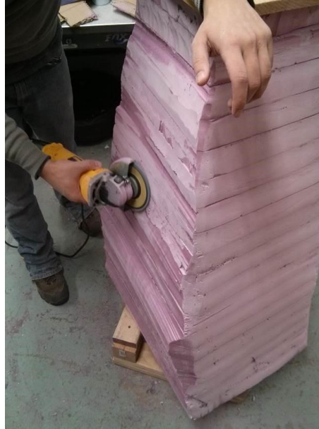
Figure 143: Sanding with the Grinder
