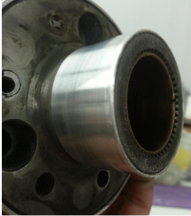
Figure 90: Shaft Bushing Pressed into Place
