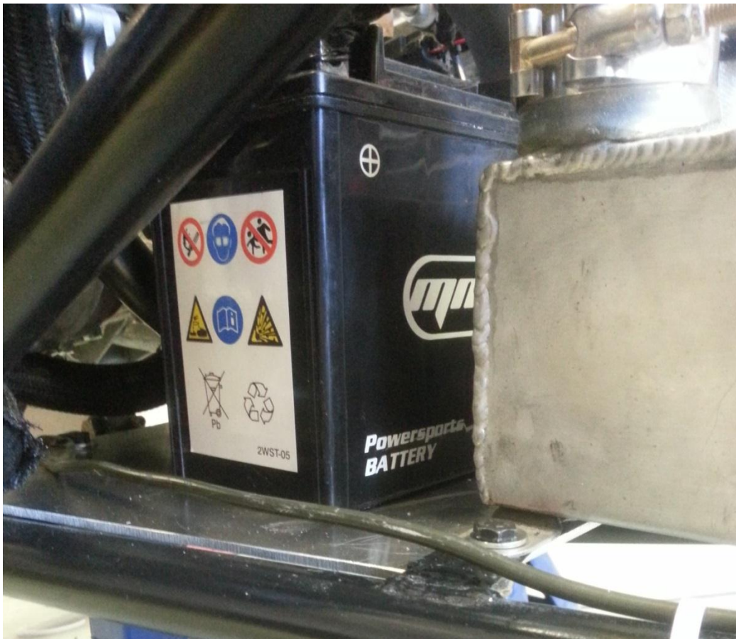
Figure 127: Installed Battery (Side View)
