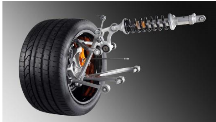
Figure 42: Example of Pushrod Suspension
