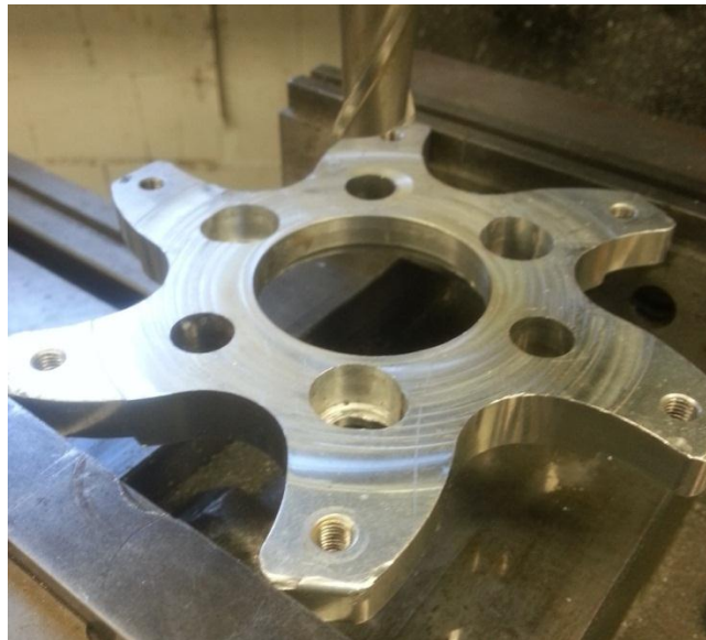
Figure 87: Sprocket Mount before Machining
