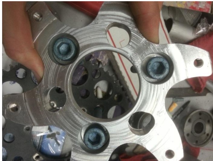
Figure 91: Sprocket Mount with New Counterbored Holes
