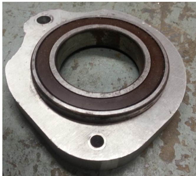
Figure 85: Old Differential Bearing
