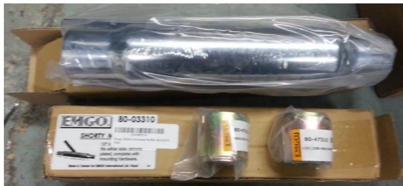
Figure 157: The Two Mufflers and Two Reducers
