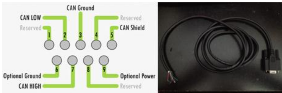
Figure 118: Male 9 Pin D-Sub Connector
