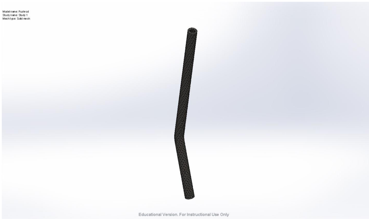
Figure 48: Pushrod without Rib Mesh
