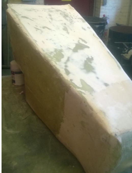
Figure 152: Filled Surface Defects
