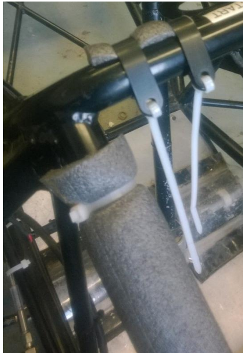
Figure 154: Frame Foam and Mounting Position
