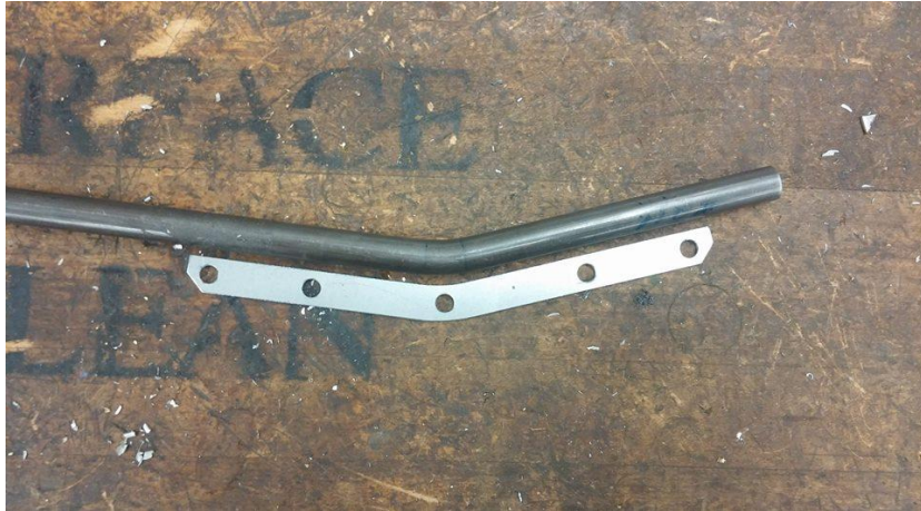
Figure 58: Machined Pushrod and Rib
