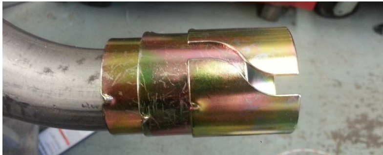
Figure 158: Reducer on the Header Pipe
