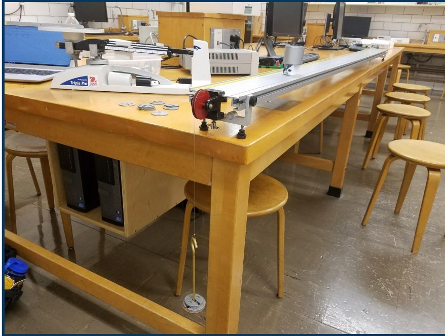
Figure 12: Coefficient of Static Friction Test Setup
