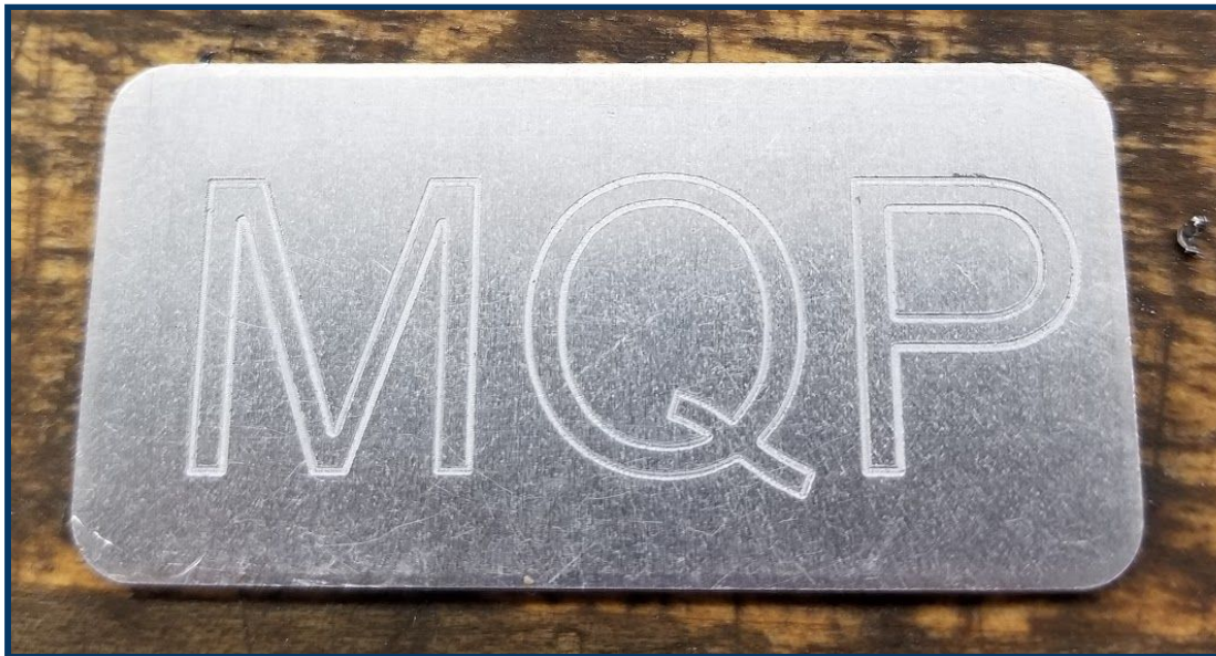
Figure 13: Finished Engraving Operation
