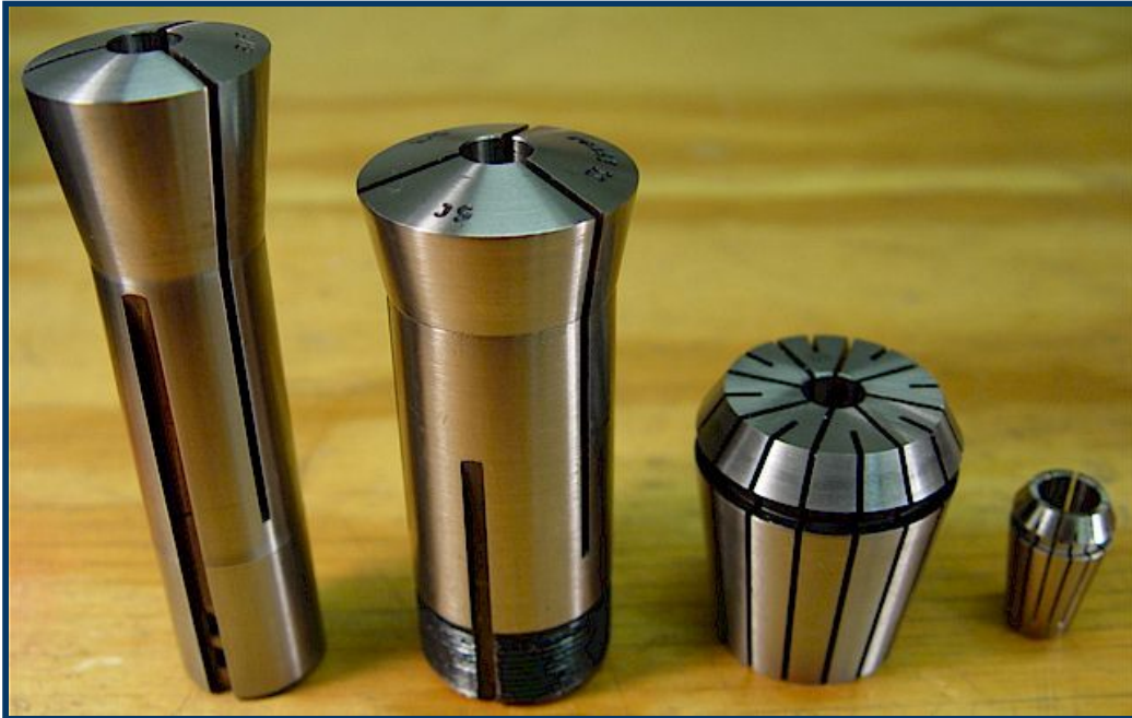
Figure 3: Four Different Styles of Collets [5]
