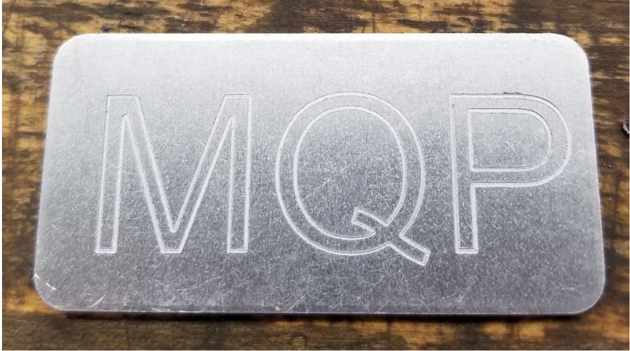
Figure 23: Business Card - Engraving Proof of Concept - Finished Part
