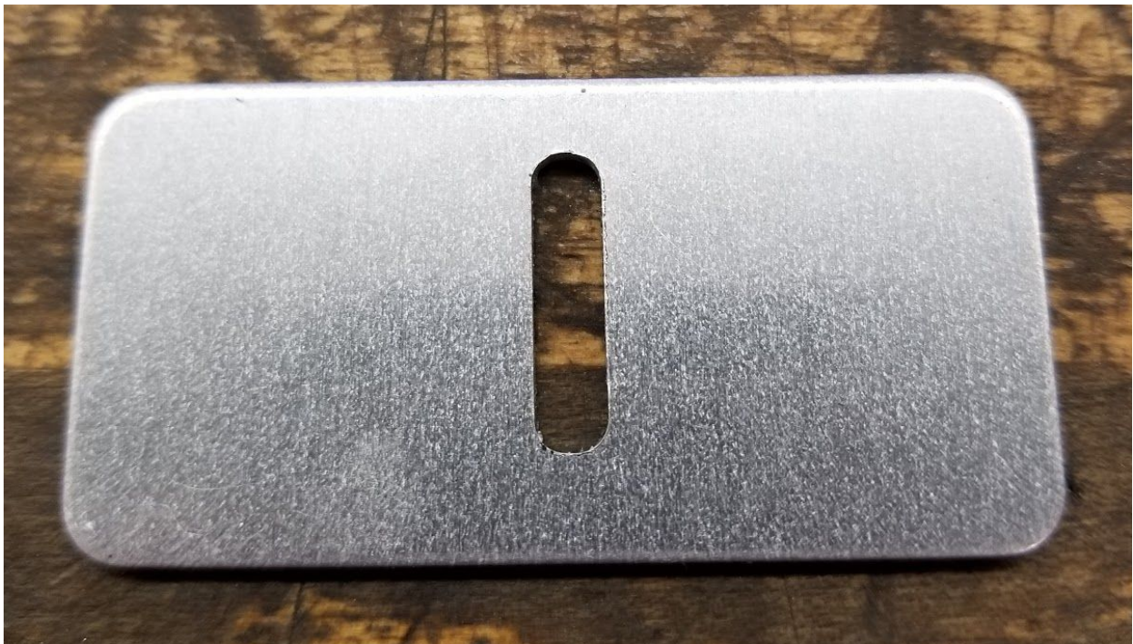
Figure 24: Business Card - Pocket Through Test - Finished Part
