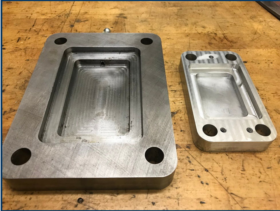
Figure 27: A comparison of our first fixture plate design (left) and our final fixture plate design (right)
