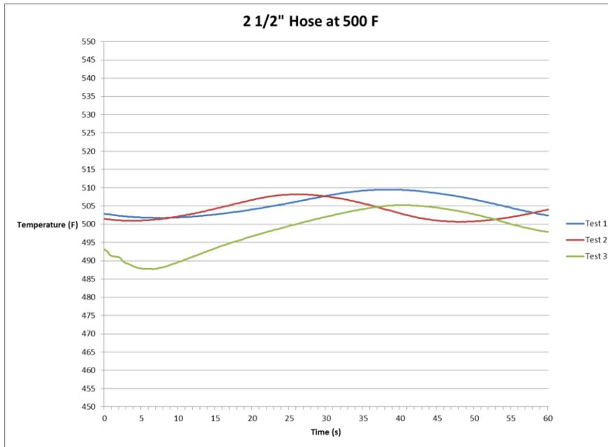
**Figure 18: 2 1/2" Hose at 500° F Temperature Data**
