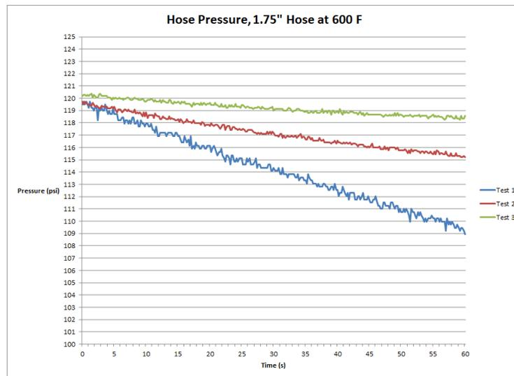
Figure 13: 1 3/4" Hose at 600° F Pressure Data
