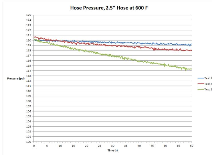
**Figure 15: 2 1/2" Hose at 600° F Pressure Data**
