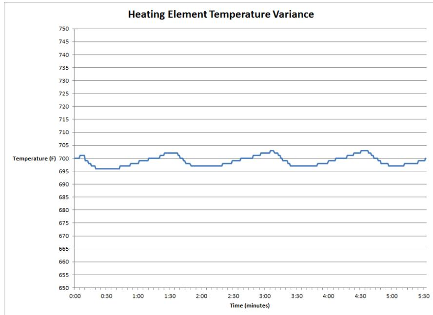
**Figure 10: Heating Element Verification Test Temperature Data**
