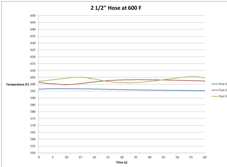
**Figure 19: 2 1/2" Hose at 600° F Temperature Data**
