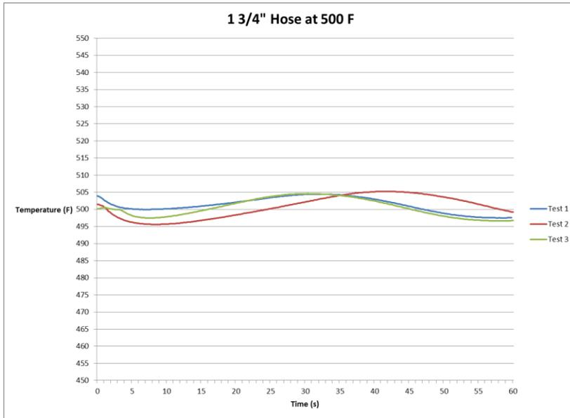
Figure 16: 1 3/4" Hose at 500° F Temperature Data
