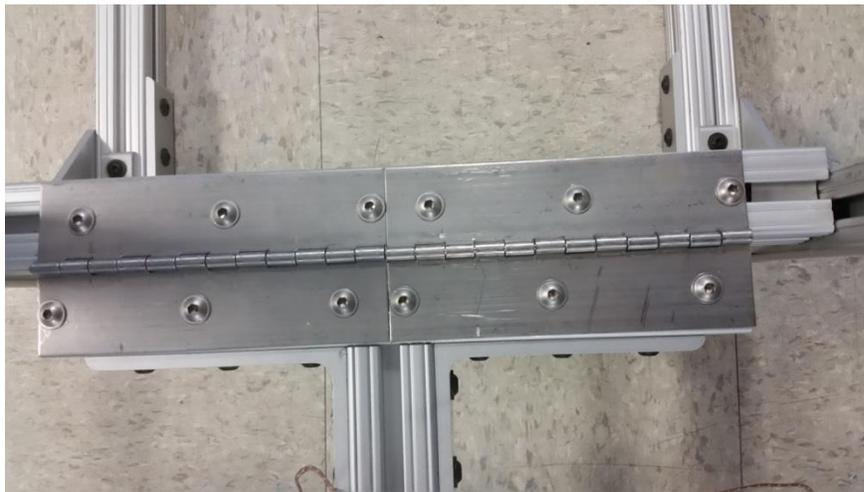
Figure 3: Top-down View of Hinges
