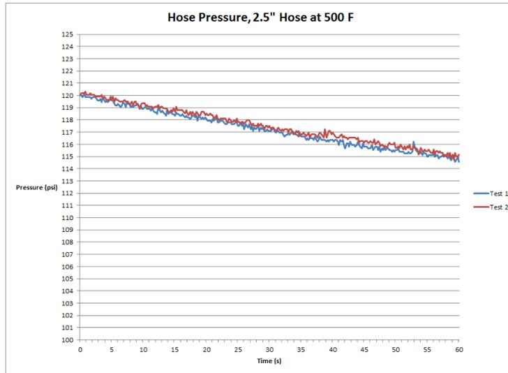
**Figure 14: 2 1/2" Hose at 500° F Pressure Data**
