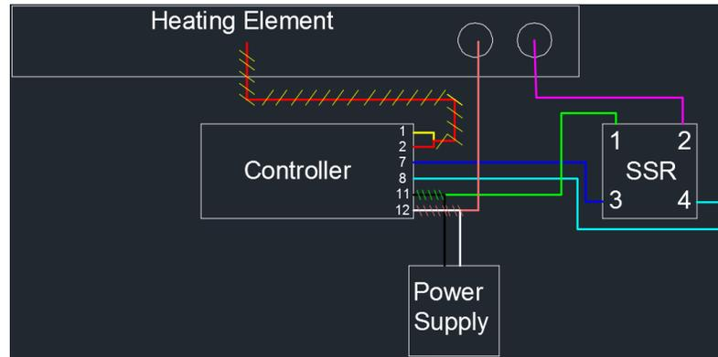
Figure 9: Wiring Diagram
