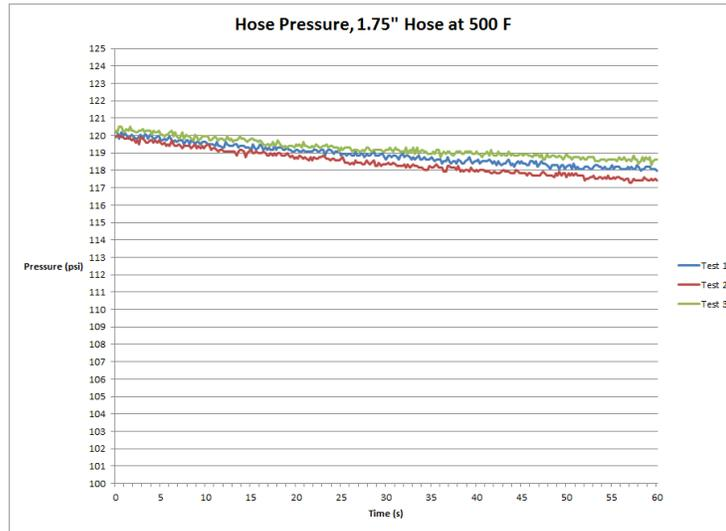
Figure 12: 1 3/4" Hose at 500° F Pressure Data
