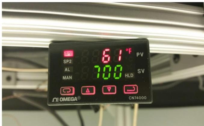
Figure 8: PID Controller
