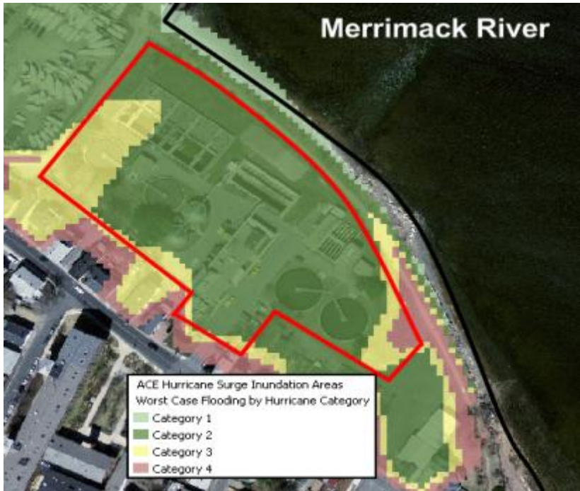
ACE Hurricane Surge Inundation Area map for the Newburyport Wastewater Treatment Plant
