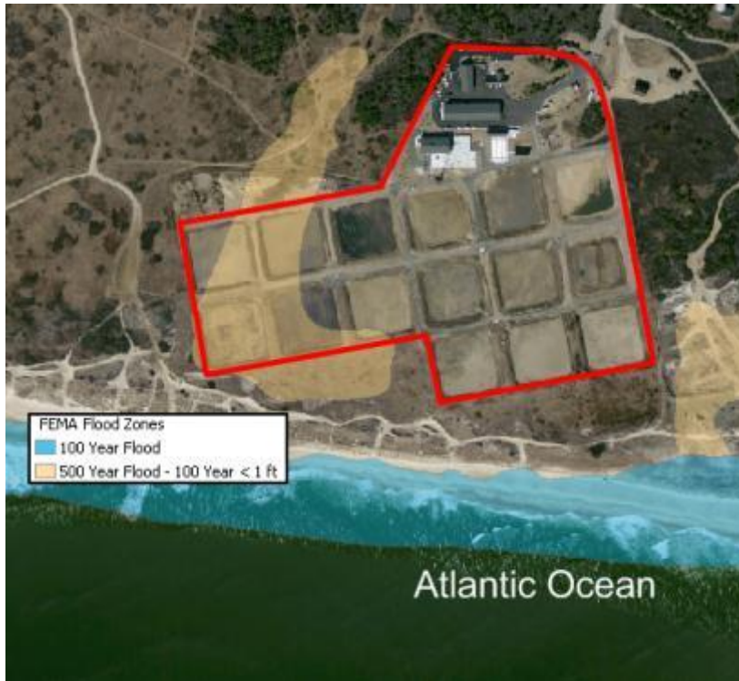
FEMA Flood Zone map for the Nantucket Wastewater Treatment Facility. The red line indicates the boundary of the facility. (500 year flood – 100 year <1 ft is the combination of the 500 year flood zone and 100 year flood zone under one foot)
