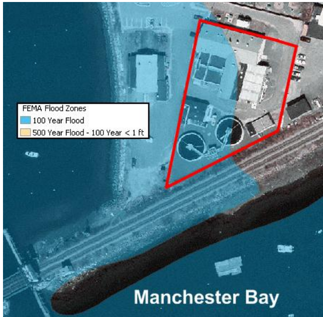
FEMA Flood Zone map for the Manchester Wastewater Treatment Plant. The red line indicates the boundary of the facility. (500 year flood – 100 year <1 ft is the combination of the 500 year flood zone and 100 year flood zone under one foot)
