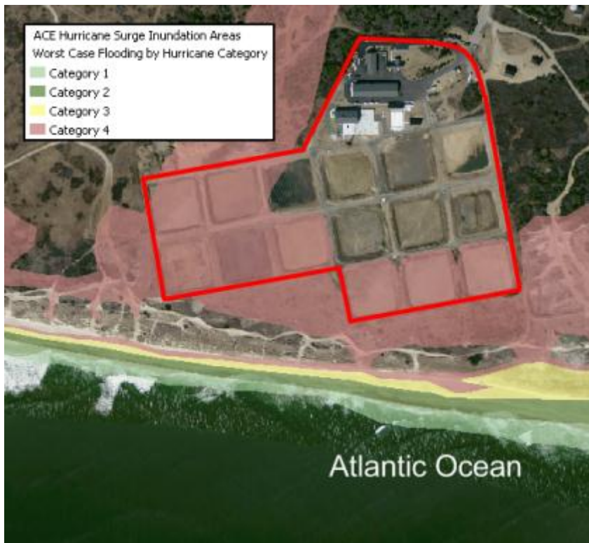
ACE Hurricane Surge Inundation Area map for the Nantucket Wastewater Treatment Facility
