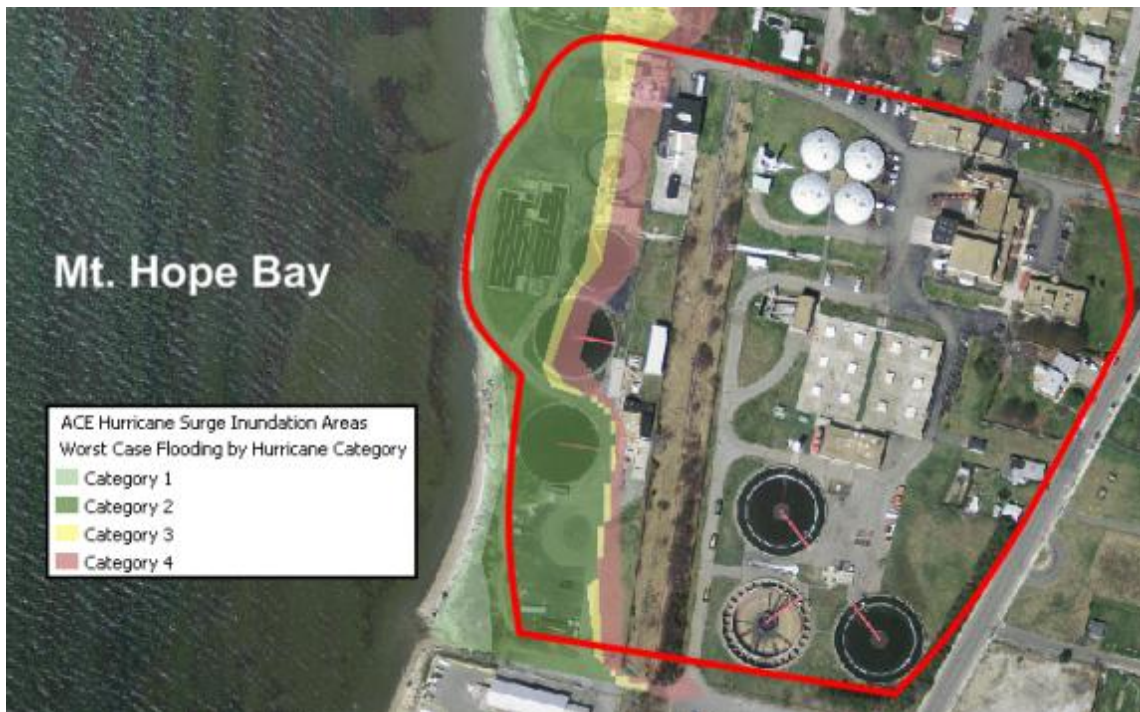
ACE Hurricane Surge Inundation Area map for the Fall River Wastewater Treatment Plant
