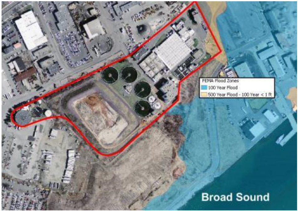
FEMA Flood Zone map for the Lynn Wastewater Treatment Plant. The red line indicates the boundary of the facility. (500 year flood – 100 year <1 ft is the combination of the 500 year flood zone and 100 year flood zone under one foot)
