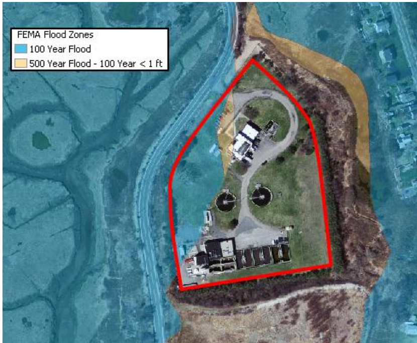
FEMA Flood Zone map for the Marshfield Wastewater Treatment Facility. The red line indicates the boundary of the facility. (500 year flood – 100 year <1 ft is the combination of the 500 year flood zone and 100 year flood zone under one foot)
