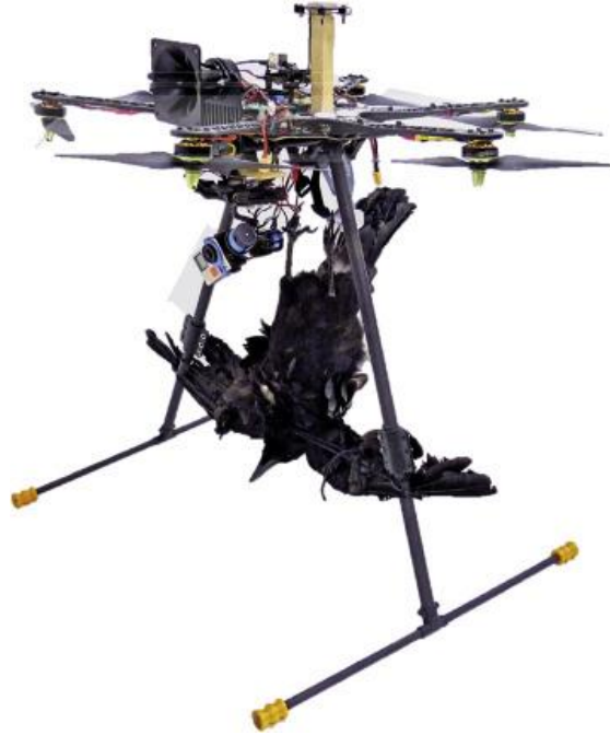
Figure 8: A bird-repelling UAV carrying a taxidermy crow [16]
