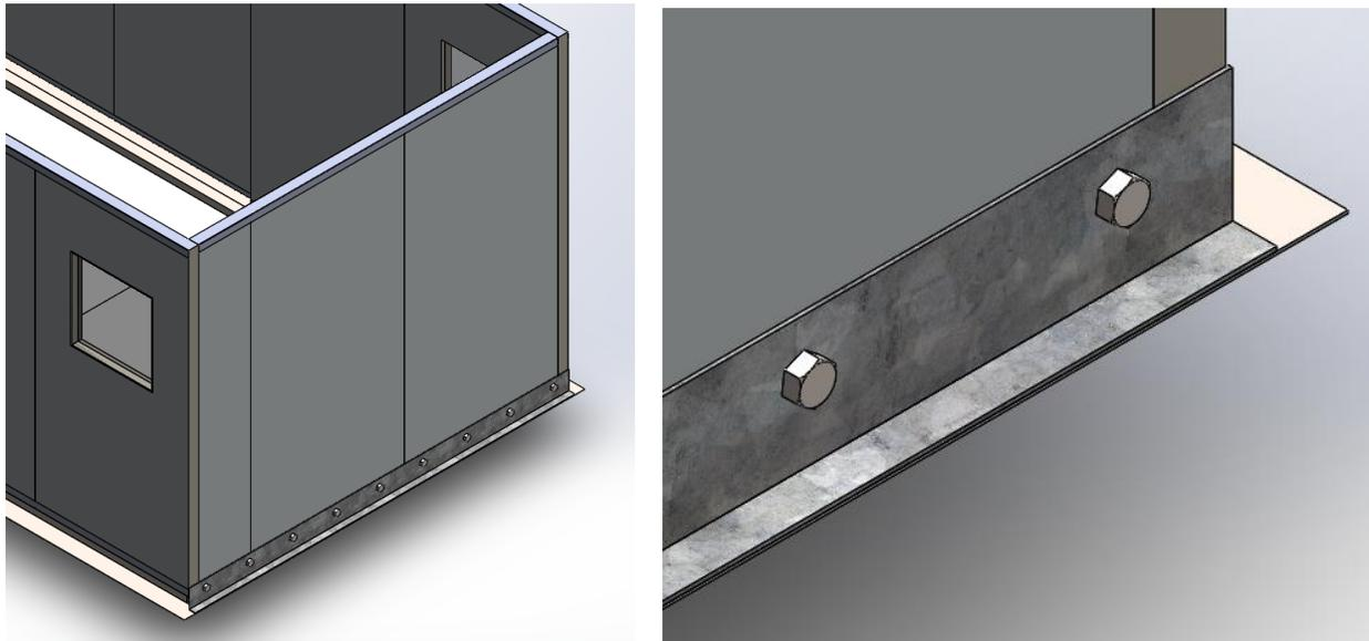
*Figure 54: Locking mechanism*
