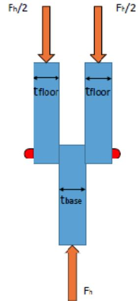
The Shear and Bearing Stress can be calculated as shown for double shear. Using these values, a Safety Factor was determined using the yield strength of the material.
