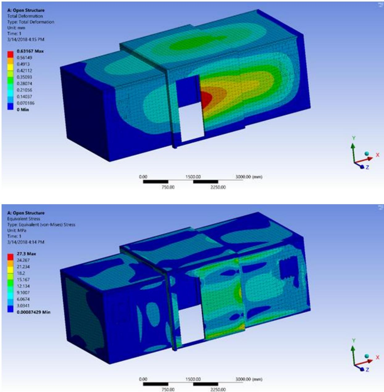
Figure 48: Deformation and Stress (146 mph wind)
