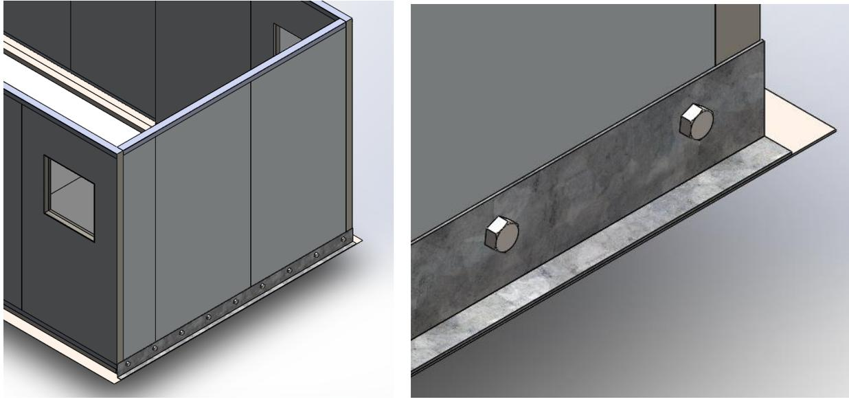
Figure 34: Locking mechanism
