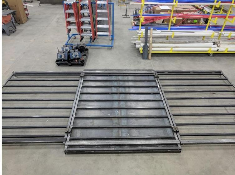
*Figure 67: Assembled floor frame*
