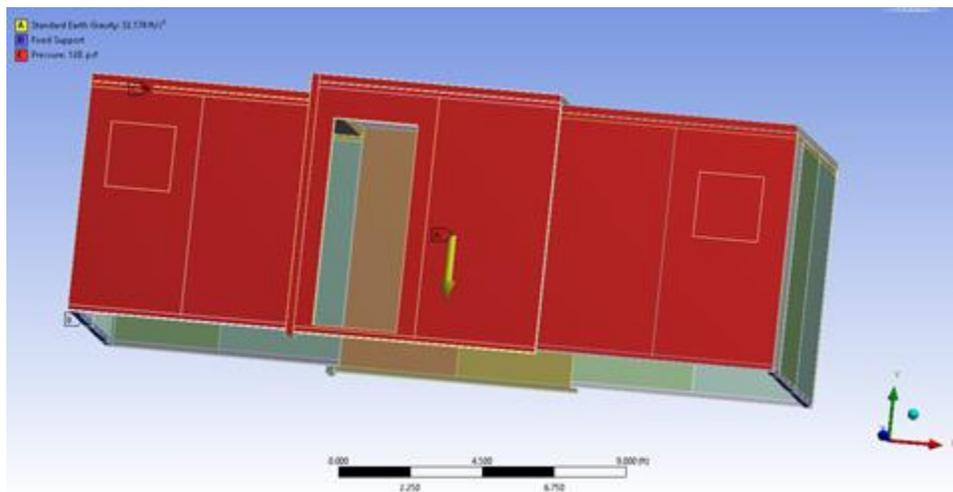
Figure 45: Model set-up for wind load analysis
