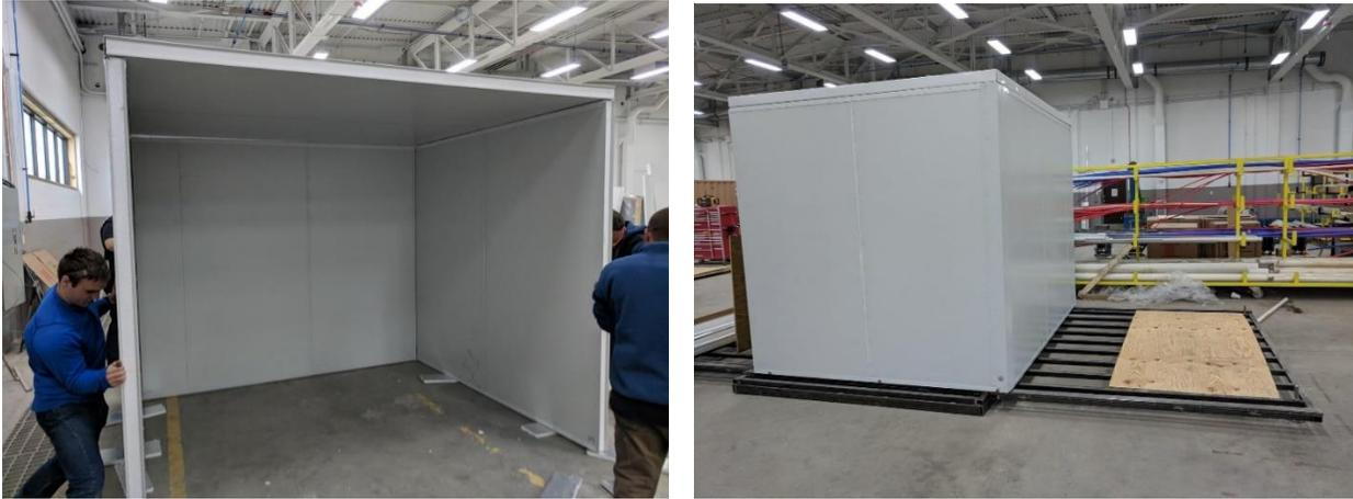
*Figure 69: Medium compartment wall and roof assembly*
