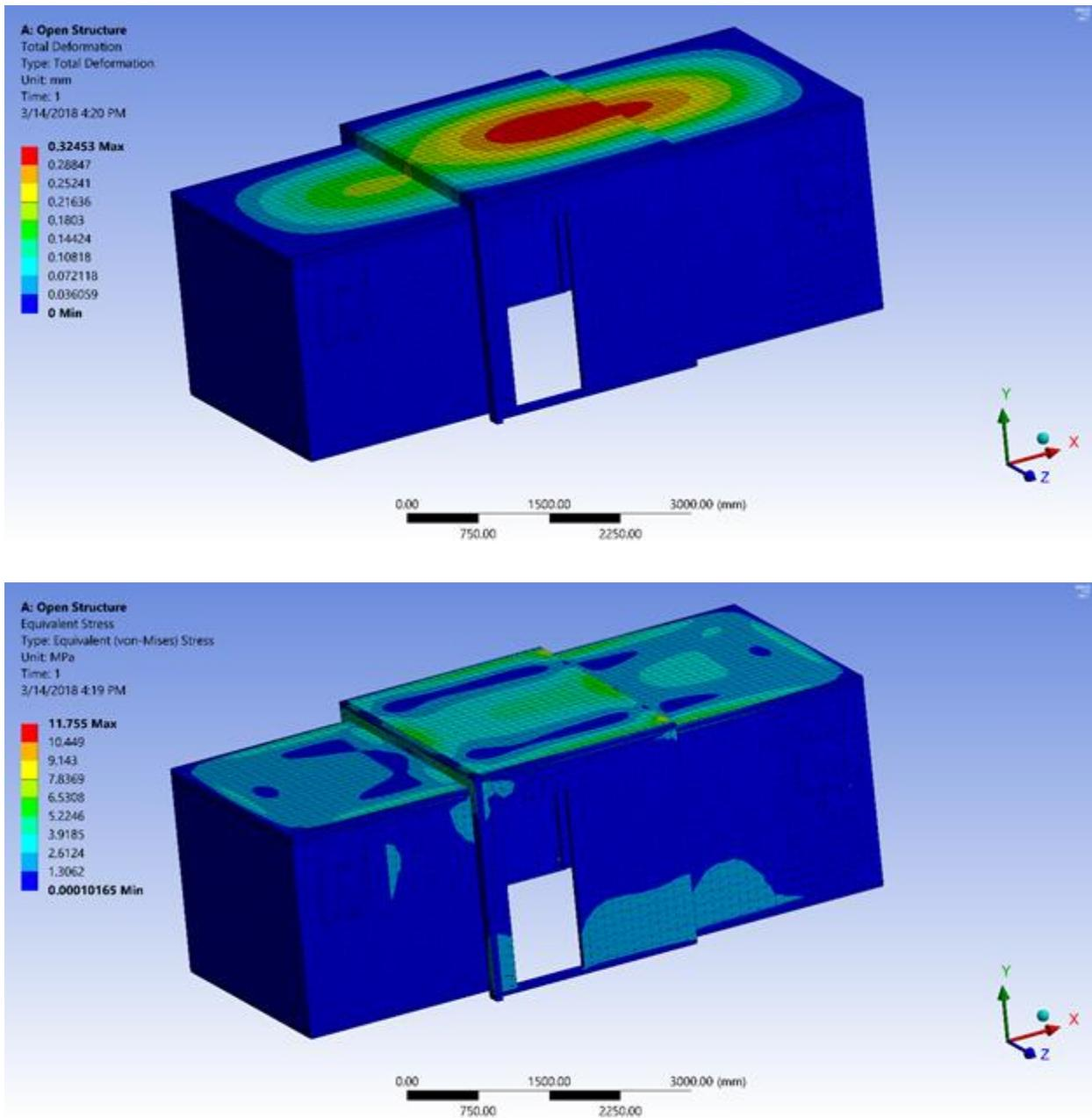
Figure 46: Deformation and Stress (9 mph wind)
