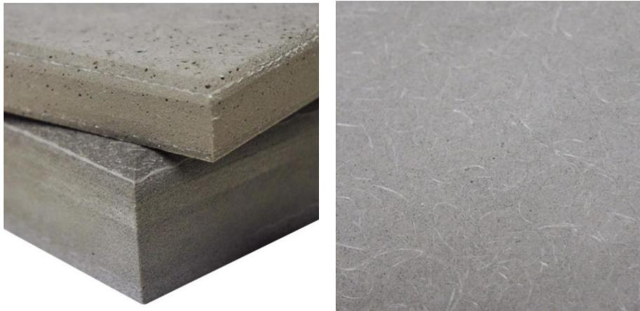
Figure 27: Coosa Board composite floor with close-up of fiberglass reinforced plastic (right)
