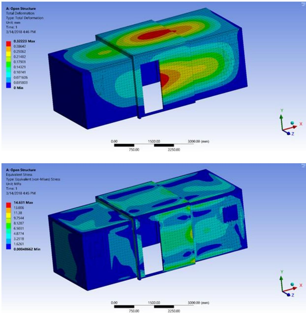
Figure 47: Deformation and Stress (110 mph wind)
