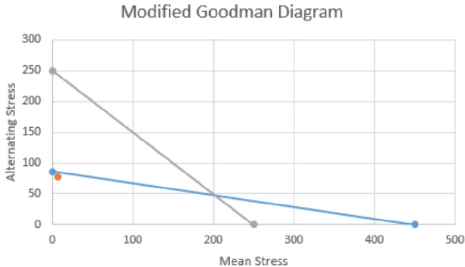
Figure 59: Modified Goodman Diagram [MPa] - 110 mph
