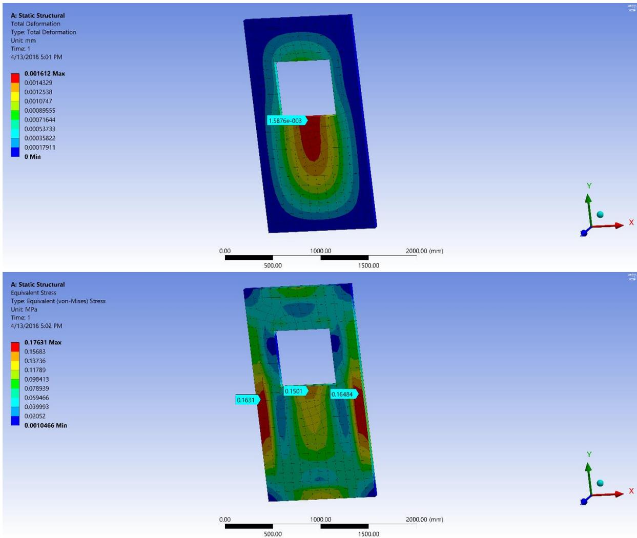
Figure 40: Measured stress and deformation values, 100 mm mesh
