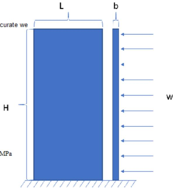
The distributed load comes from the pressure on the panel due to the wind
