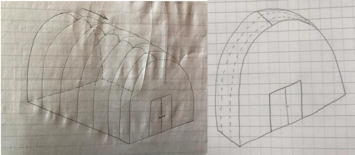
Figure 7: The Accordion Design, expanded (left) and collapsed (right)
