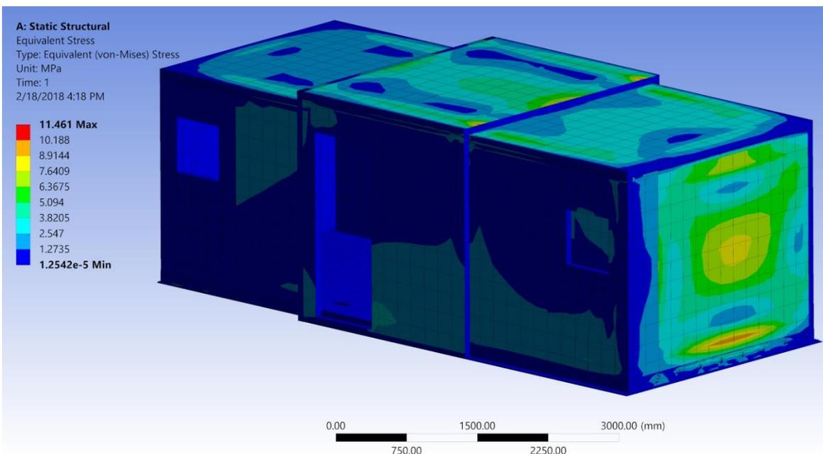
Figure 44: Deformation and Stress, 146 mph wind (small face)
