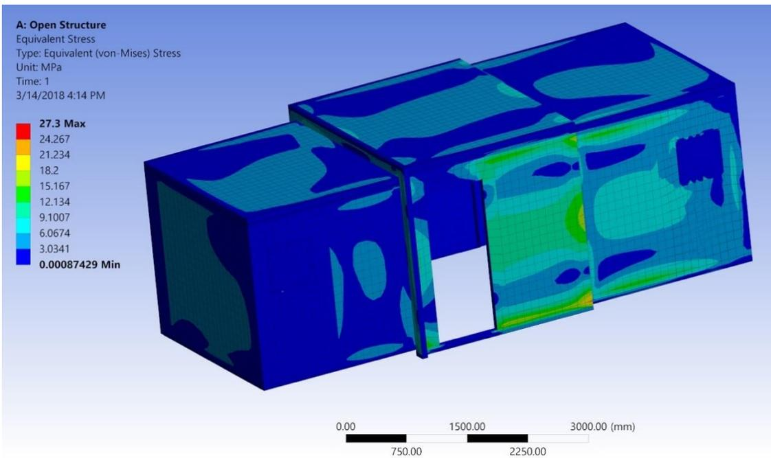
Figure 42: Deformation and Stress, 146 mph wind (large face)
