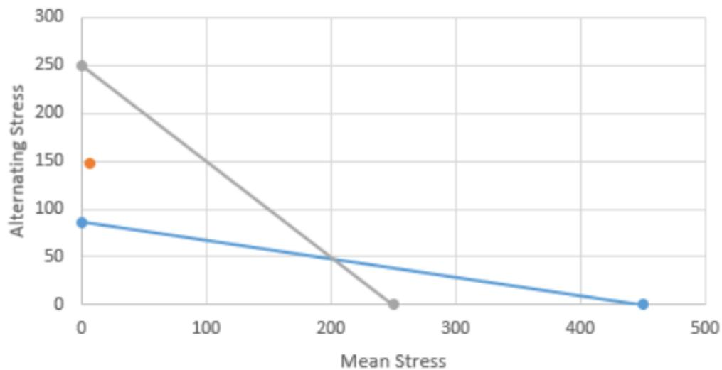
Figure 61: Modified Goodman Diagram [MPa] - 146 mph
