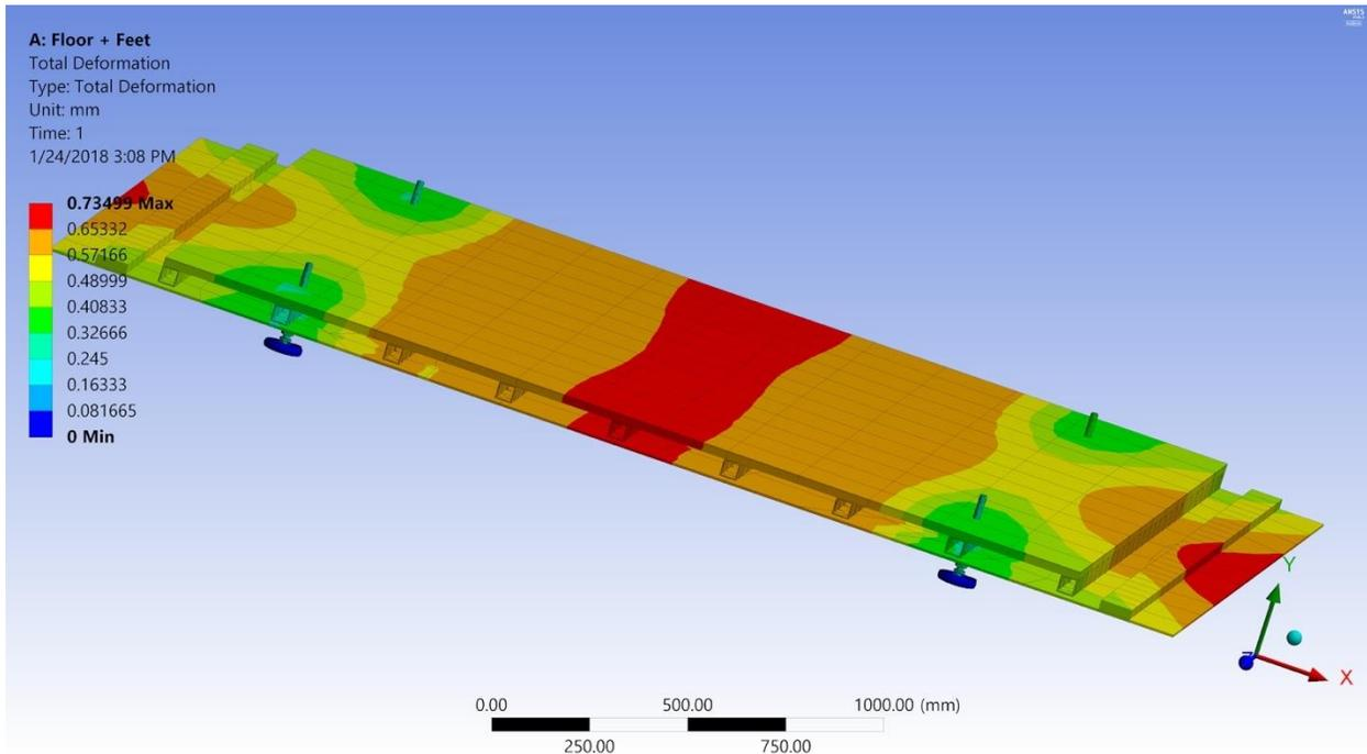
Figure 50: Floor Assembly Deformation (10,000 lb distributed load)
