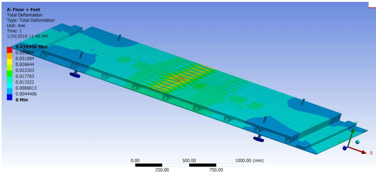
Figure 51: Floor Assembly Deformation (200 lb point load)
