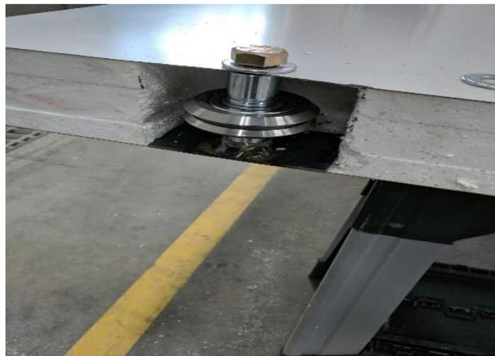
*Figure 68: V-Track wheel assembly*
