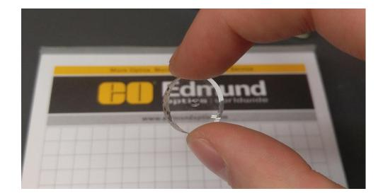
Figure 17: Core/cladding sample showing the difference between the undoped outside region and doped core (spot in the center showing reflection).
