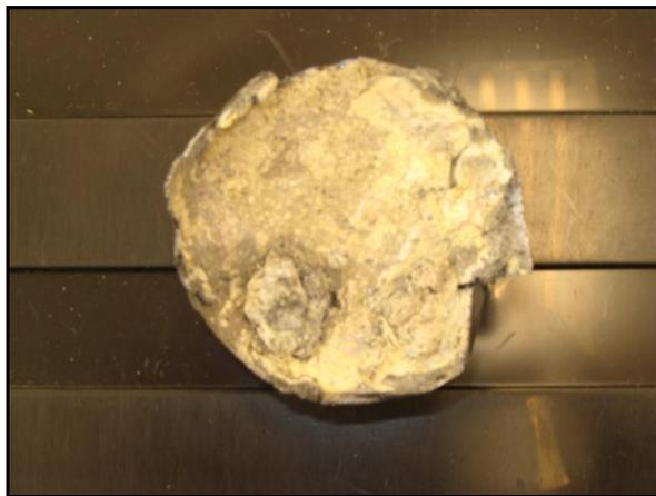
**Figure 17: Yellowish layer of magnesium nitrides on the surface of the casting**
