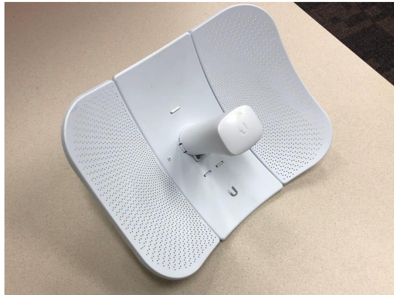
Figure 3.10. Ubiquiti LBE-5AC-GEN2-US Base Station Dish
