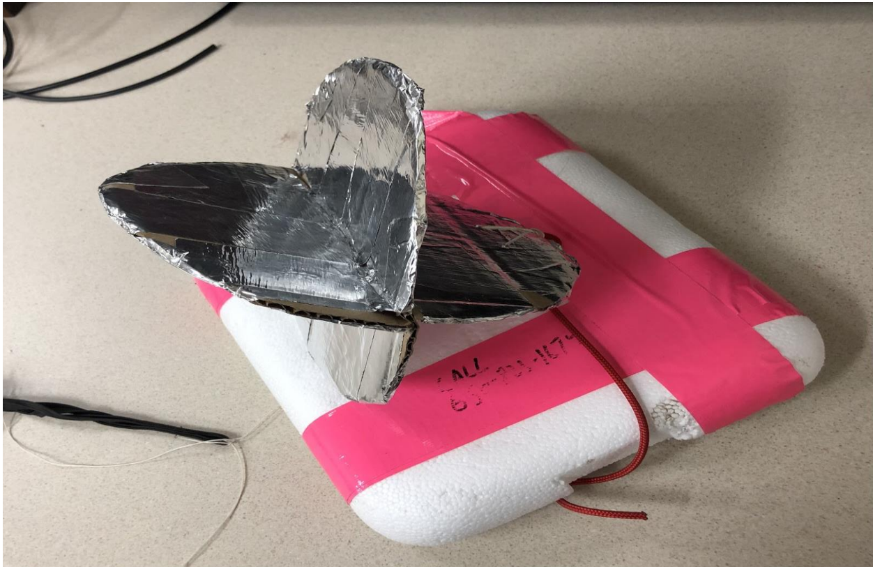
Figure 3.1. The radar reflector which we constructed and attached to our HAB. The radar reflector was made using pieces of cardboard and aluminum tape.
