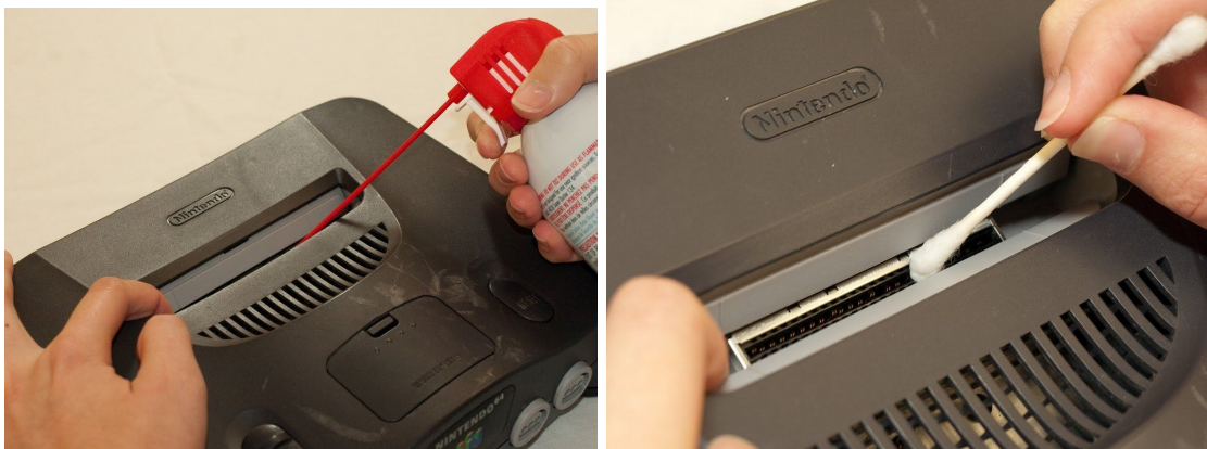
Figure 33: Air Dusting The N64 Cartridge Slot 82 Figure 34: Swabbing The N64 Cartridge Slot 83
