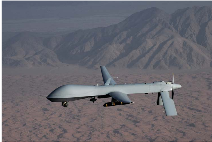
Figure 1.3: The MQ-1 Predator Unmanned Aircraft, an Unmanned Aerial Vehicle requiring multiple operators[2]
