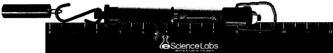
Figure 7: Step 3 reference. Notice that the end of the free spring is lined up to the 0 cm mark of the ruler.
