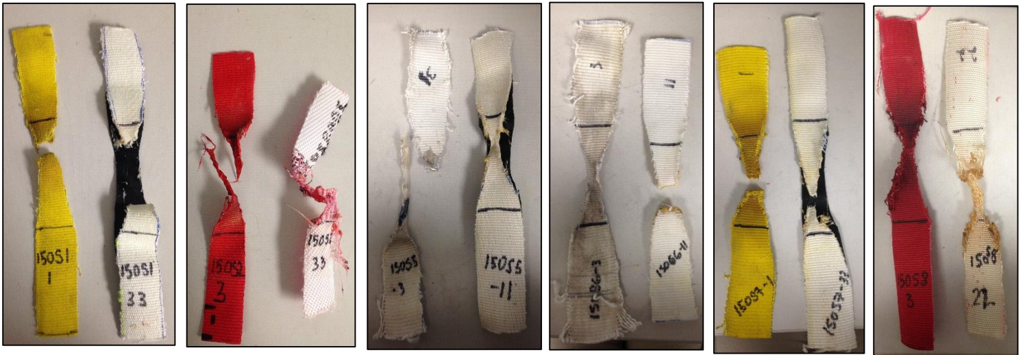
Figure 11: Hoses 1-6 After 150°C Testing. Outer Jackets on Right, Inner Jackets on Left
