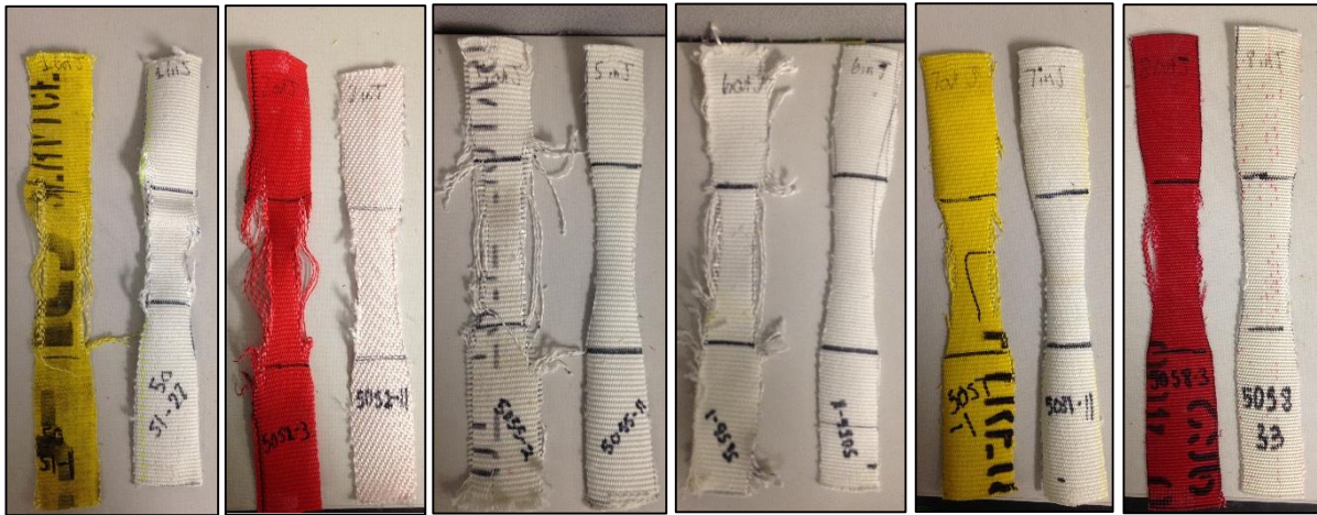
Figure 8: Hoses 1-6 After 50°C Testing. Outer Jackets on Right, Inner Jackets on Left
