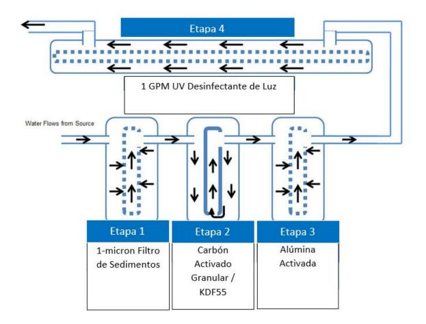
Figure 12: A visual representation of the flow of water through each stage of filtration.
