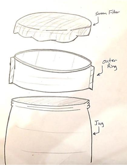
Figure 19: Exploded View of the Screen Filter Assembly
