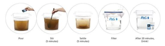
Figure 32: The Full Process of Purifying Dirty Water (P&G Demonstration, (n.d.))
