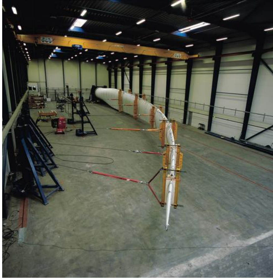
Fig. 4.8 Turbine Blade Static Testing (EWEA, 2011)
