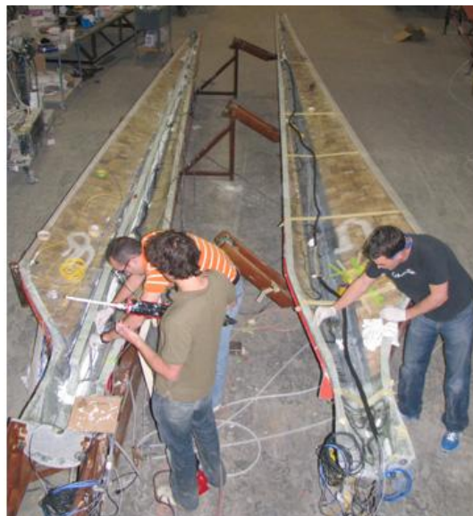
Fig. 4.7 Embedded Sensor Installation in Turbine Blades (Sandia, 2011)
