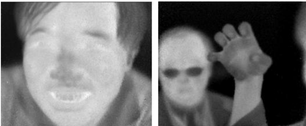
Figure 2-7. Representative thermal images obtained using reference subtraction and computer post processing of data from a MEMS thermomechanical IR detector [21].
