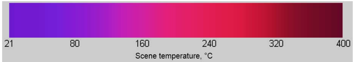
Figure 7-16. Representation of the gamma corrected color output from the reflectometry based direct viewer as calculated from measured linear RGB values.
