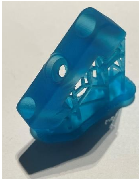
Figure 39: Resin printed 2-leg part for pin-on-disk tribometer.
