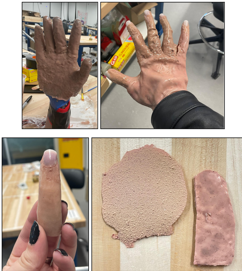
Figure 47: The top two pictures show the first and second iterations of the hand portion of the glove. The bottom left shows what a finger could look like if we were able to get a proper casting of the hand. The bottom right includes pictures of the multiple steps taken to create the skin.
