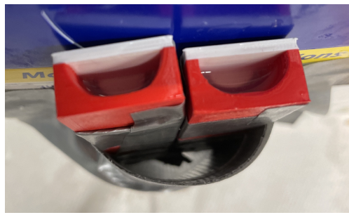
Figure 36: Finger molds curing vertically
