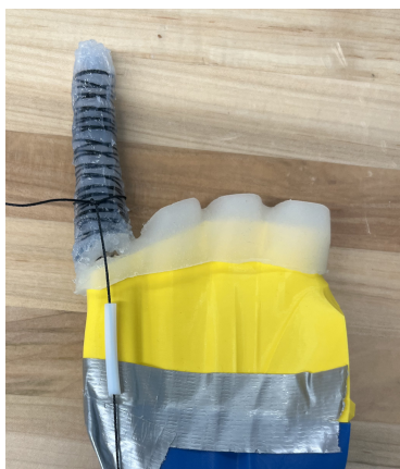
Figure 40: Cable guide positioned before glued into place
