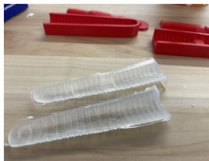
Figure 37: Finger halves removed from mold
