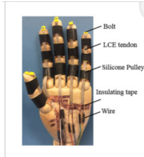
Figure 3: liquid crystal elastomer (LCE) and liquid metal (LM) prosthetic hand. Reproduce from [19]
