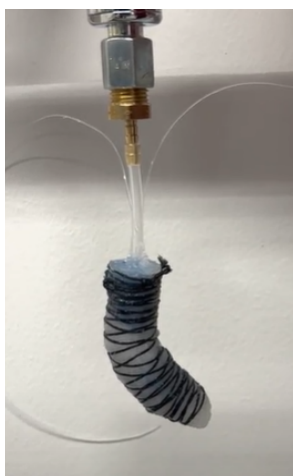
Figure 27: Fully assembled thumb actuating using positive pneumatic pressure
