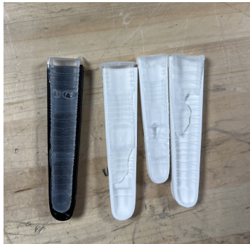
Figure 35: Failed finger molds
