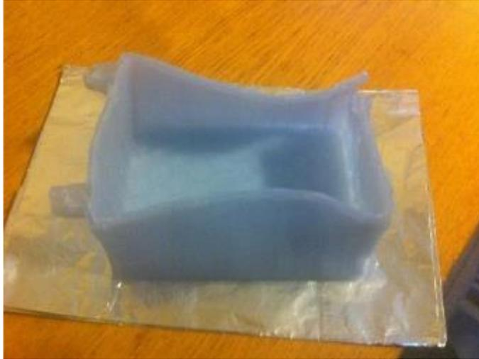
Results: Feels as though it is rubber, it seems like its hardening. Still no strand deformation or melting.
