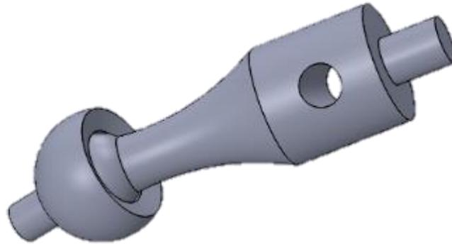
*Figure 31: CAD model of the 3-D printed ball and socket joint*
