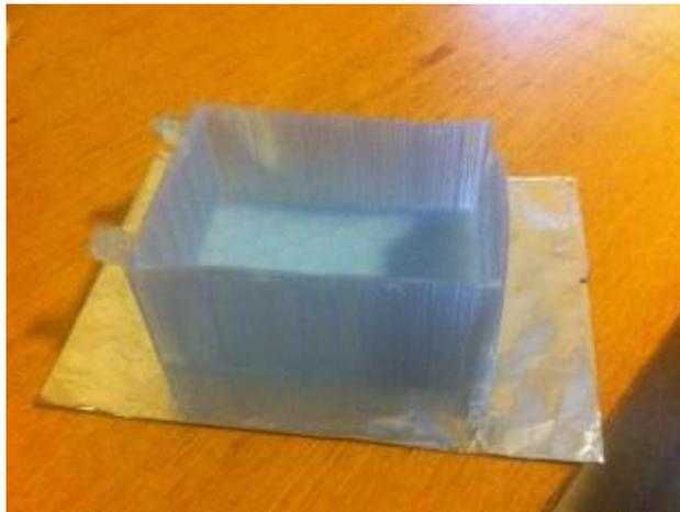
Results: PLA becomes malleable, outlying pieces and center walls can be bent up, however the corners are still rigid. (The wall that was bent slightly from the previous test, flattened back out when it was heated up.)
