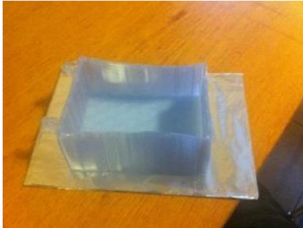
Results: Highly malleable center walls, corners are still fairly rigid, there is no melting or strand deformation.
