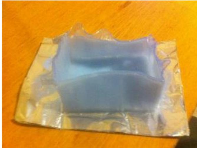
Results: Similar to previous test, strand deformation can occur if force is applied to the melted area. Transparency remains, there is still no charring.
