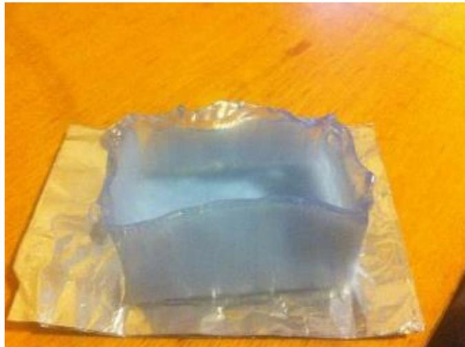
Results: more melting that previous test, strand deformation can occur more easily. Base has begun to melt in a few areas. It is becoming malleable again.
