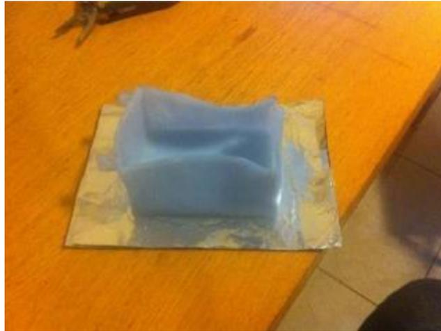
Results: Becoming rigid, very center of walls can be bent, but corners are sturdy and Very slight melting at broken corner. Strand deformation can occur on the melted area.
