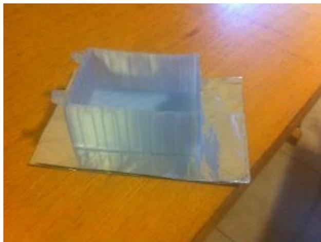
Results: Highly malleable center walls, corners became unstable, no melting or strand deformation.
