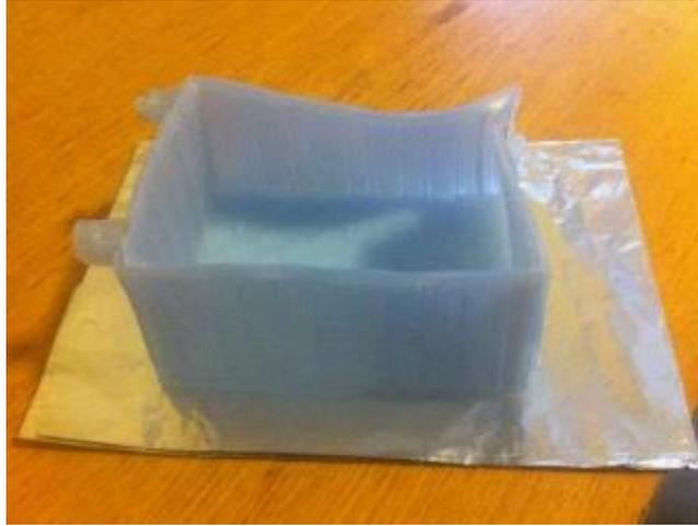
Results: Highly malleable structural integrity seems to be diminishing, it feels as though I could ball it up, but there is not melting and no strand deformation.
