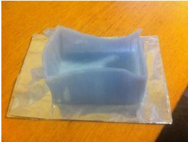
Results: Similar to previous test is getting slightly less malleable. No melting or strand deformation.
