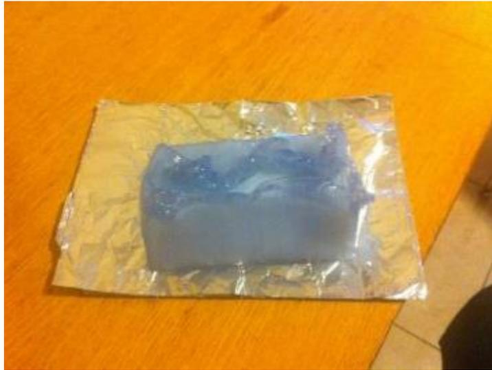
Results: Extreme melting, part of the box collapsed (the side closest to the heat source). Structural integrity is completely lost as the side melted to the base.
