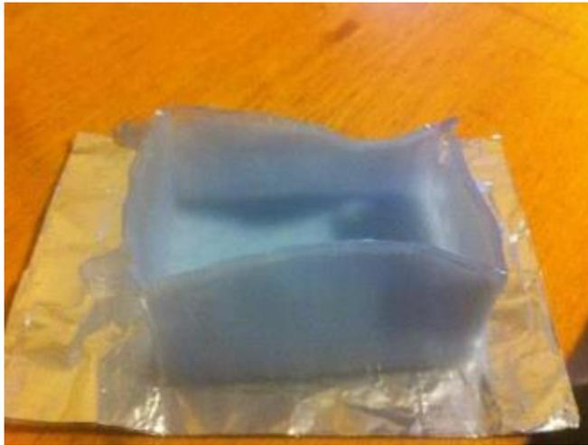
Results: Melting is occurring; the spots that have melted are now transparent. When touching the walls, the ribs are easy to feel. The melted parts are transparent after cooling. The strand deformation can occur on the melted area.
