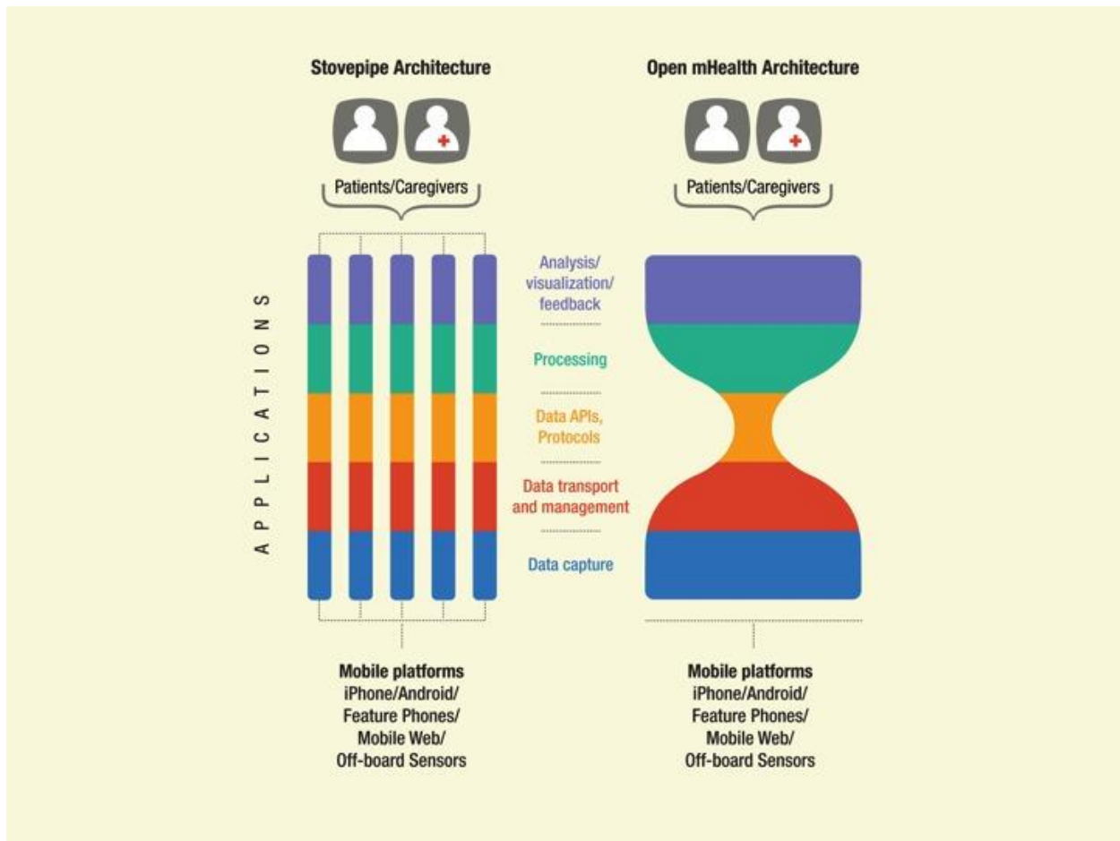
Figure 4: Diagram of Structure of Siloed (Stovepipe) Approach vs. Open mHealth
