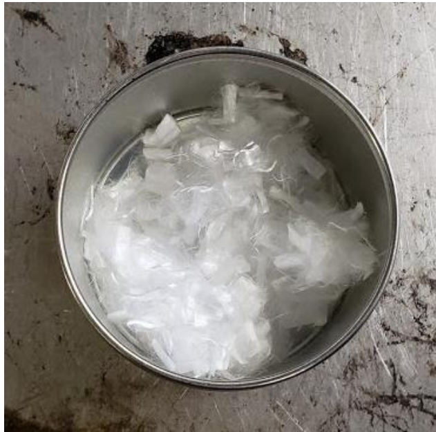
Figure 17: PPHT Fibers for 0.25% Sample Before Mixing
