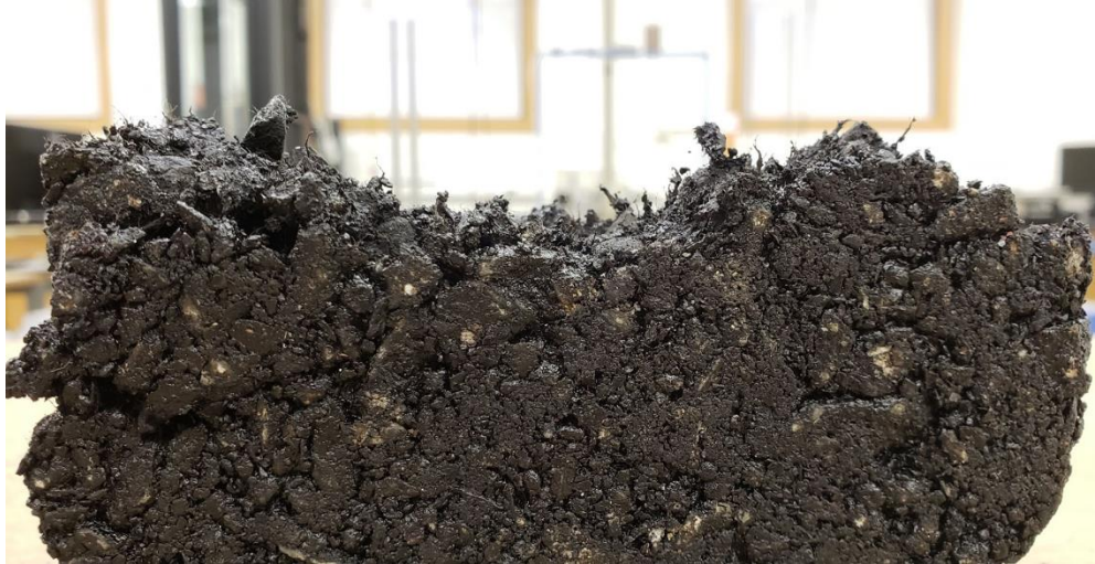
Figure 34: Fiber Sample in Half with Fibers Exposed
