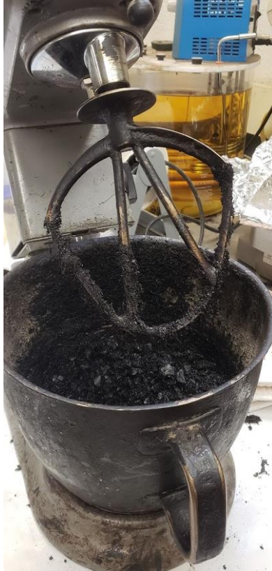
Figure 18: Asphalt-Fiber Mixture After Mixing
