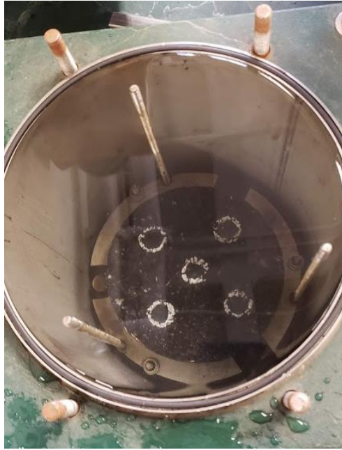
Figure 24: Sample in MIST Chamber Filled with Water
