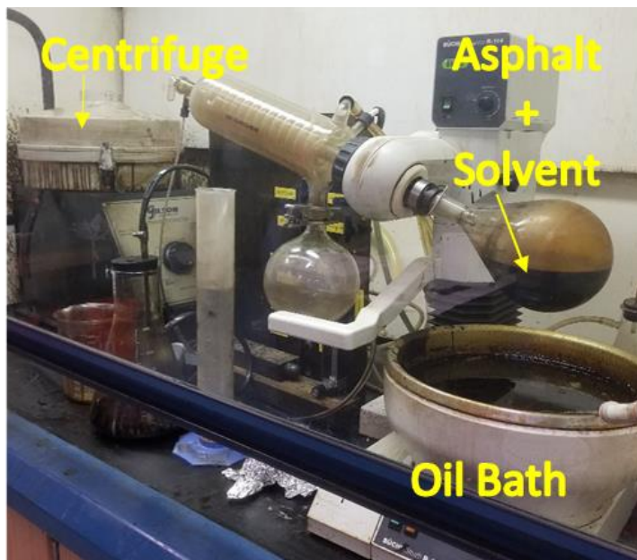
Figure 5: Binder Extraction Set-Up
