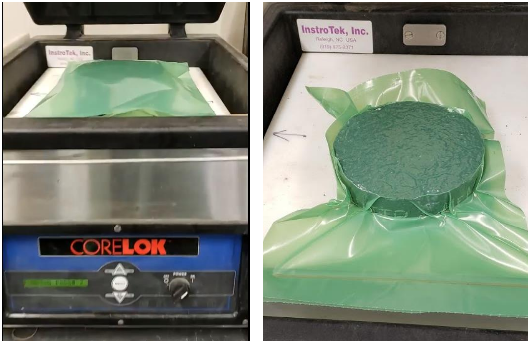
Figure 21: Sample Before and After Vacuum Sealing for Air Void Testing
