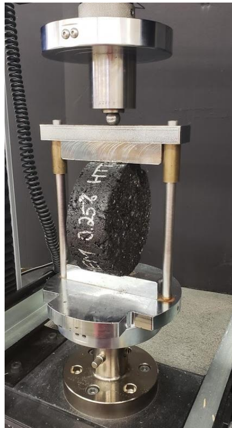
Figure 25: Sample Loaded for ITS Testing
