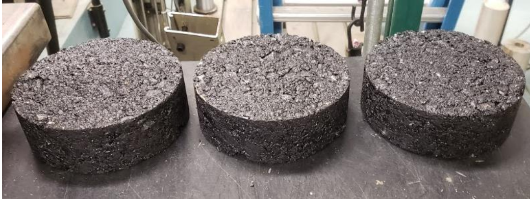
Figure 20: 0.25% PPHT Fiber Asphalt Samples After Compaction
