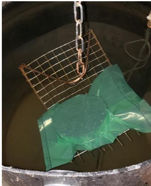
Figure 22: Sample Suspended in Water
