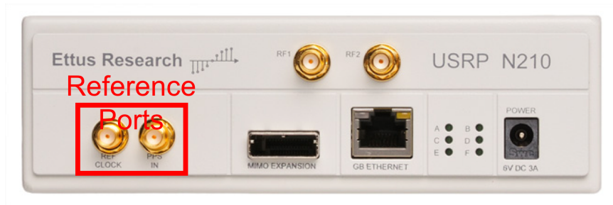
Figure 5.20: USRP-N210 from Ettus Research front panel. Consists of frequency source (REF CLOCK), clocking source (PPS IN), antenna ports (RF1,RF2), MIMO cabling input, and Gigabit ethernet.
