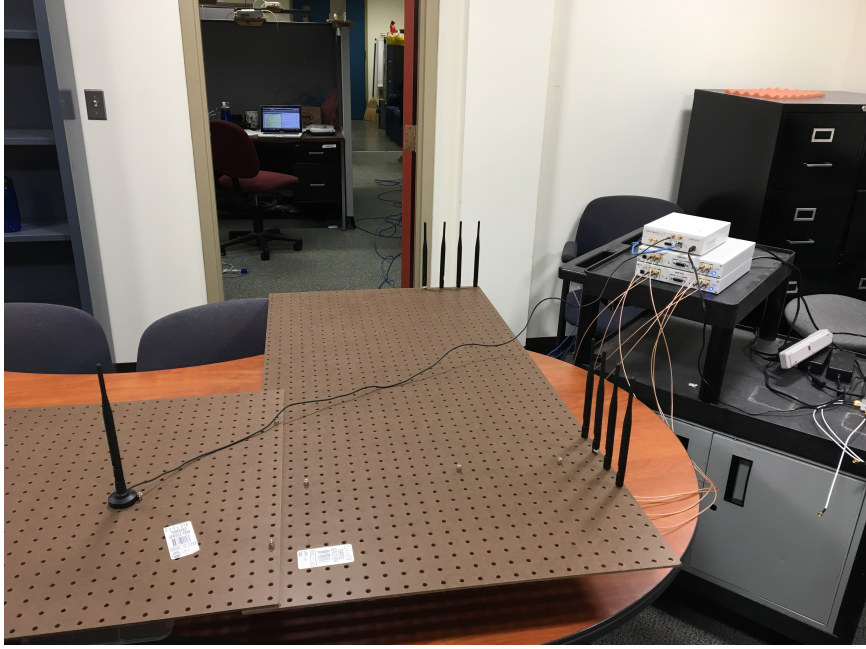
Figure 5.32: Pegboard layout of transmitter in reference to four element array. Pegboard is used to maintain accurate target positioning across azimuth.
