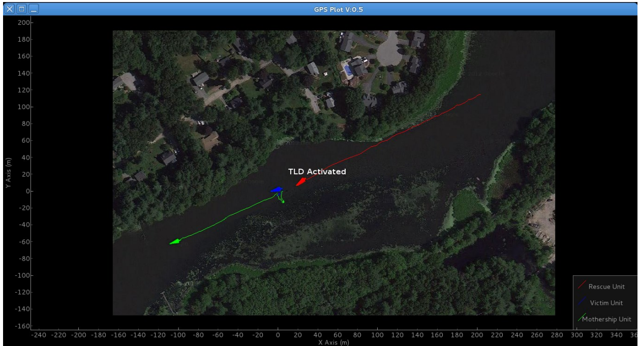
Figure 66 – Mothership GUI: Terminal locator device activated
