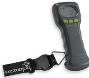
Figure 58 – Luggage Scale used to determine Drag Force on Rescue Craft (Bed Bath & Beyond, 2013)
