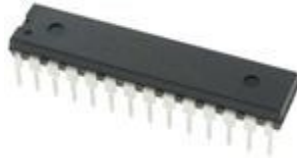
Figure 14 – Atmega 328P Microcontroller (Mouser, 2013)
