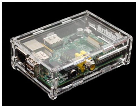
Figure 9 – Raspberry Pi enclosure
