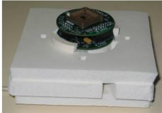
**Figure 17: Foam stabilizer, evaluation board, and sensor.**
