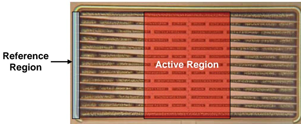
**Figure 5: Magnified photograph of a thermopile (Pillans).**
