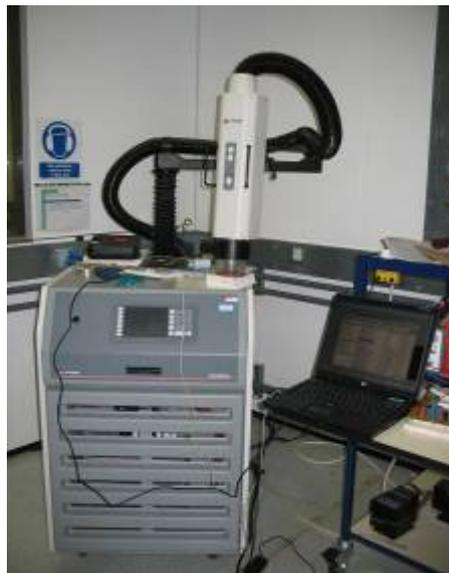
**Figure 20: Setup for the temperature cycling test.**
