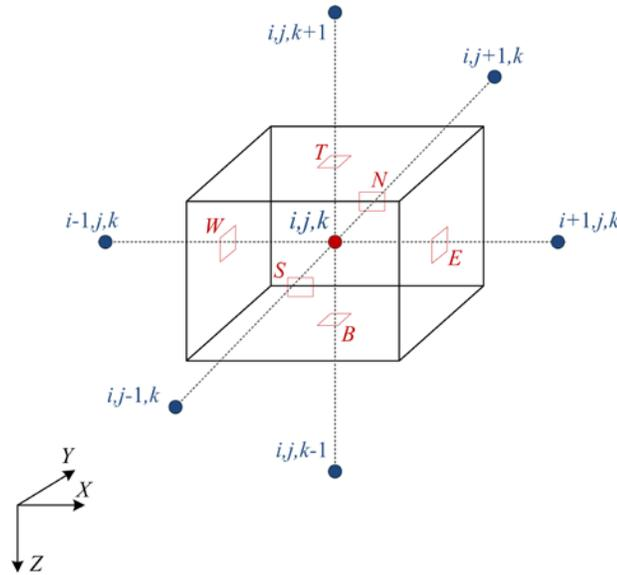
Figure 14. A finite volume at grid point  $(i,j,k)$ .
