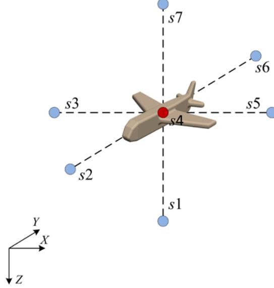
Figure 12. Example of the flying formation of UAVs for the concentration gradient measurements.
