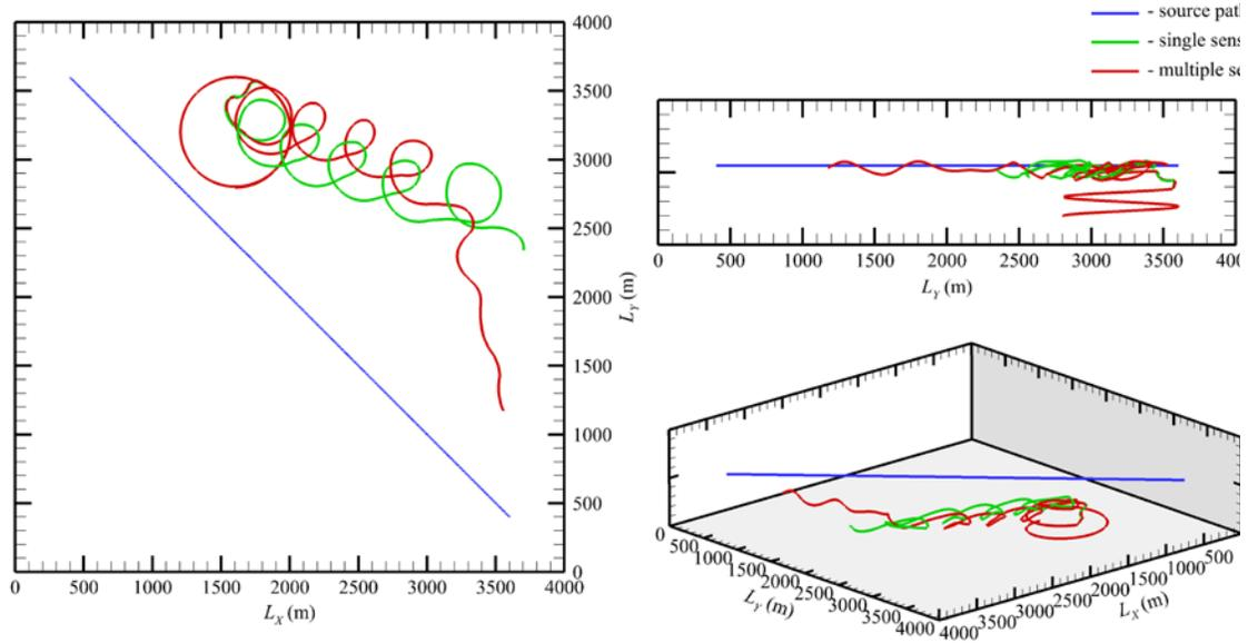
**Figure 34. Comparison of the trajectory in case of the concentration estimation with a single sensor and with multiple sensors.**
