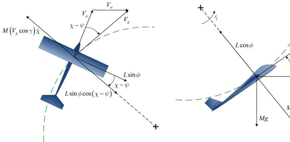
Figure 11 Free-body diagram of the forces acting on the UAV in the climbing coordinated turn: top view of the horizontal plane and side view of the vertical plane.
