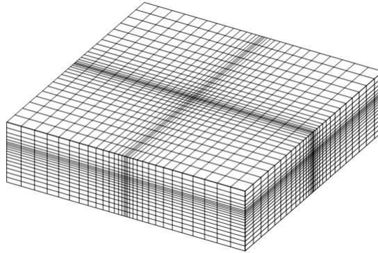
**Figure 17. Adapted nonuniform computational grid.**
