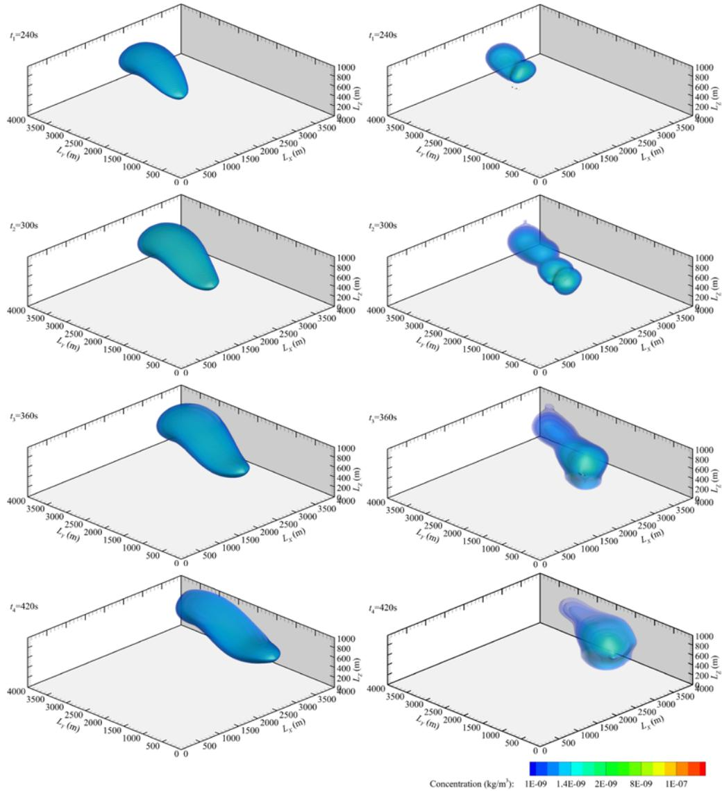
**Figure 29. Comparison between estimated plume concentration (left) and simulated concentration (right) for a source moving across the domain.**
