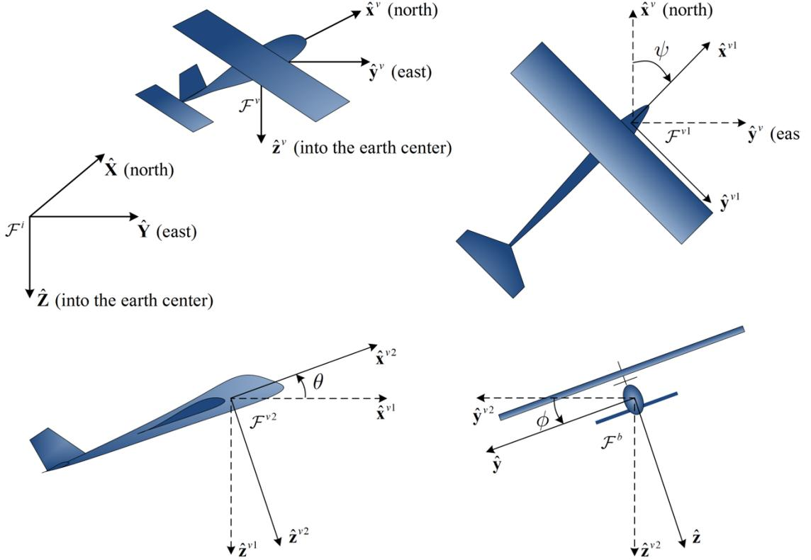
Figure 6. Transformation from the inertial frame to the body frame.
