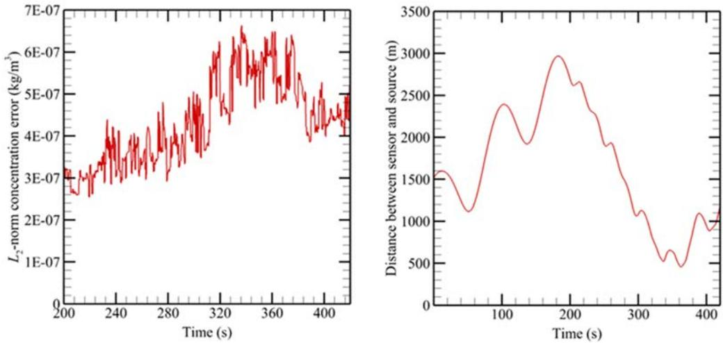
**Figure 25. Estimator performance for a moving; (Left) RMS error vs. time; (Right) distance between the UAV and the source.**
