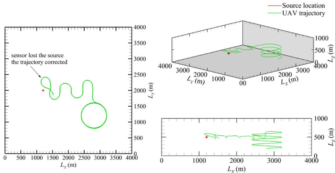
Figure 21. UAV trajectory for stationary source.
