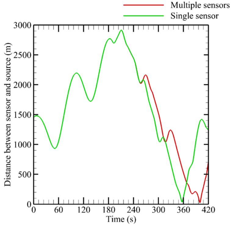
Figure 37. The distance between the sensor and source versus time for the case of a single sensor and the case of multiple sensors; the source is moving along an arc trajectory.
