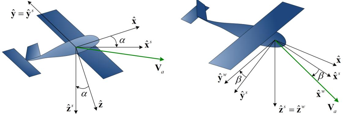
Figure 7. Transformation from the body frame to the wind frame.
