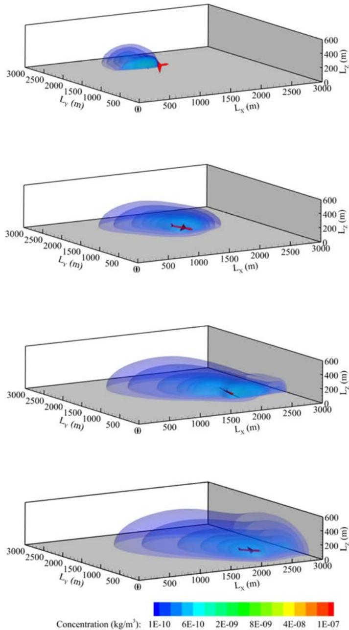
**Figure 33. Evolution of the estimated plume from 240s to 480s with 80s increments.**
