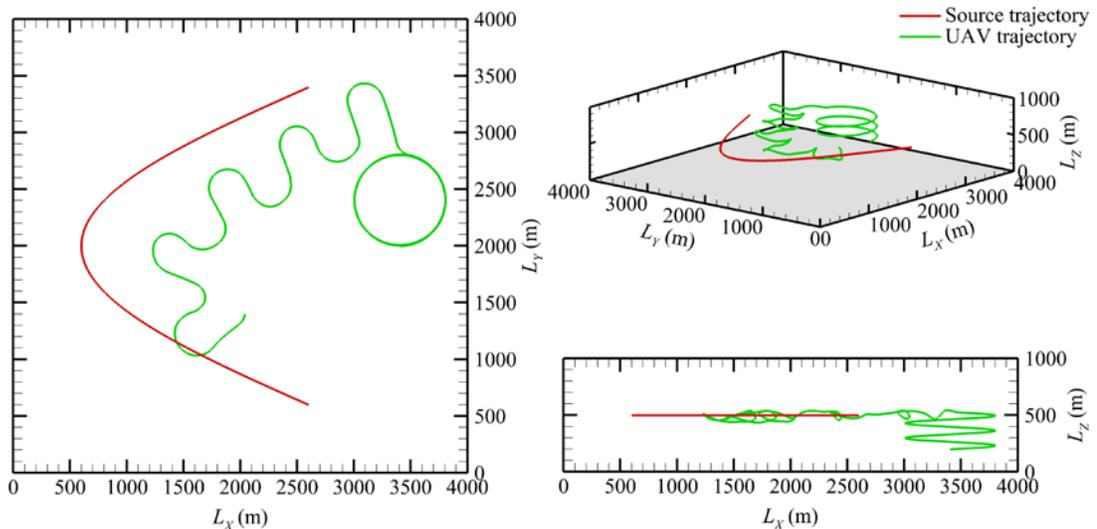
**Figure 24. UAV trajectory for a source moving along an arc trajectory.**
