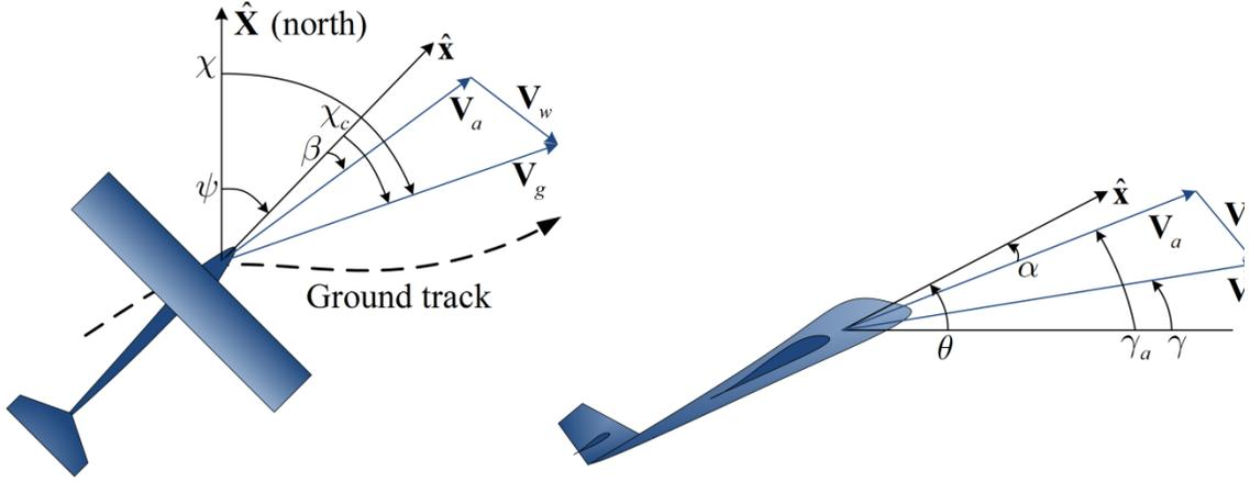
Figure 9. The wind triangle projected onto the horizontal plane (left) and vertical plane (right).
