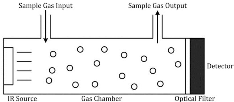
**Figure 3. IR-source gas sensor based on the basic absorption spectrometry [52]. Copyright 2012 by the authors; licensee MDPI, Basel, Switzerland**
