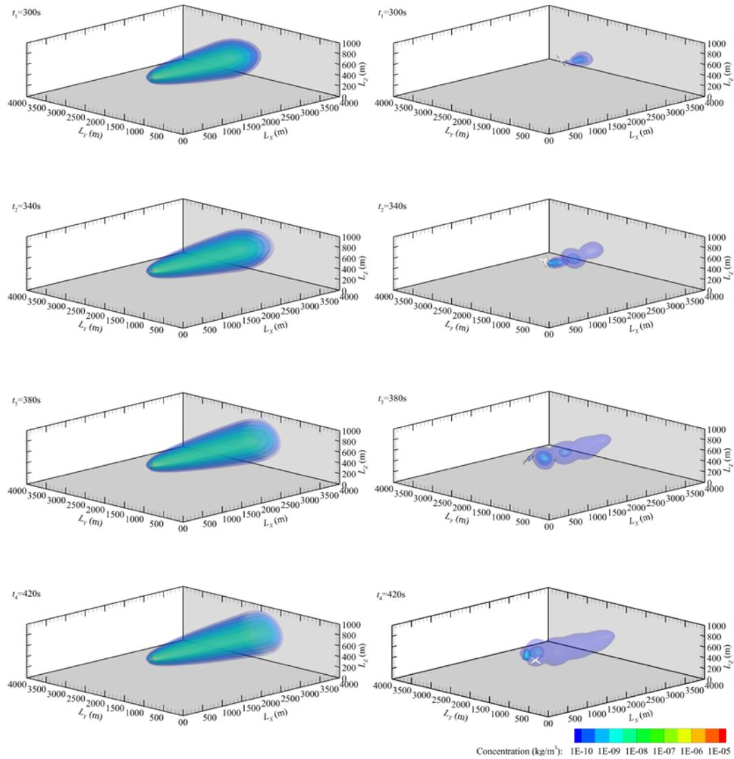
**Figure 23. Comparison between estimated plume concentration (left) and simulated concentration (right) for a stationary aerial source at various times.**
