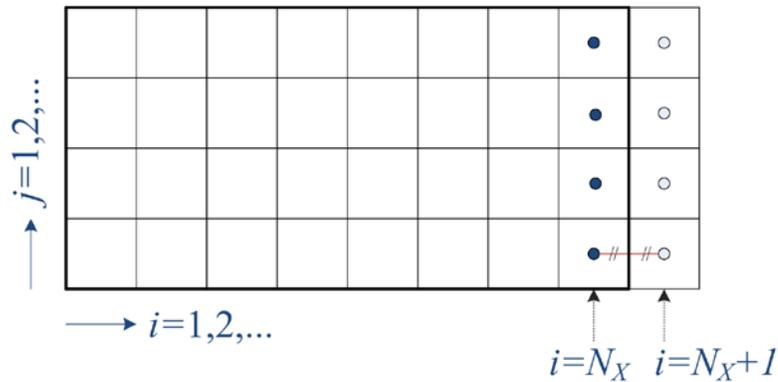
Figure 15. Finite volume discretization at the boundary.
