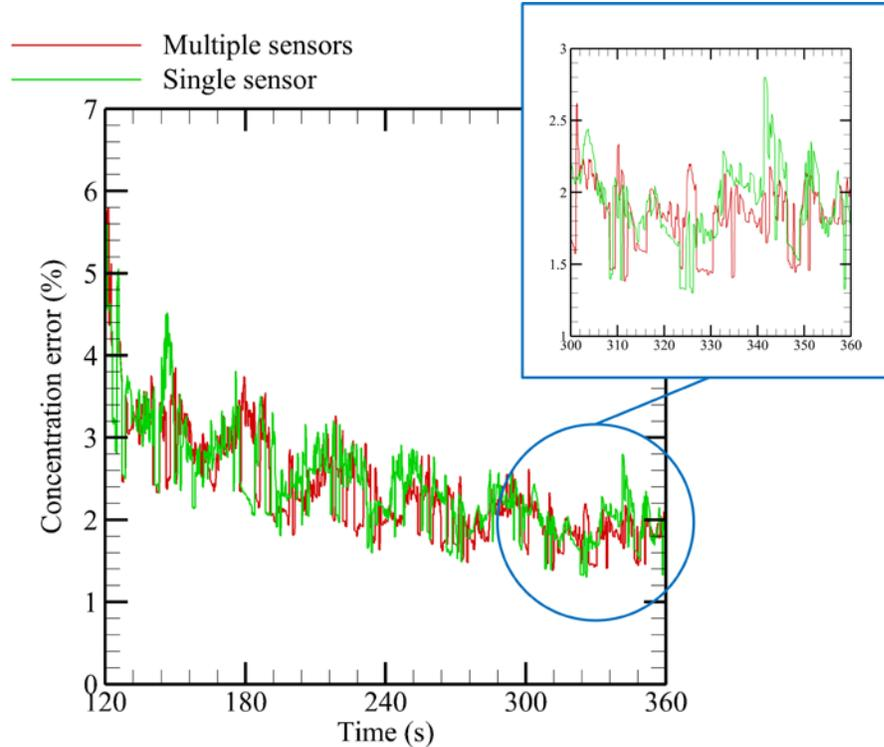
**Figure 35. The normalized concentration error versus time for the case of a single sensor and the case of multiple sensors.**
