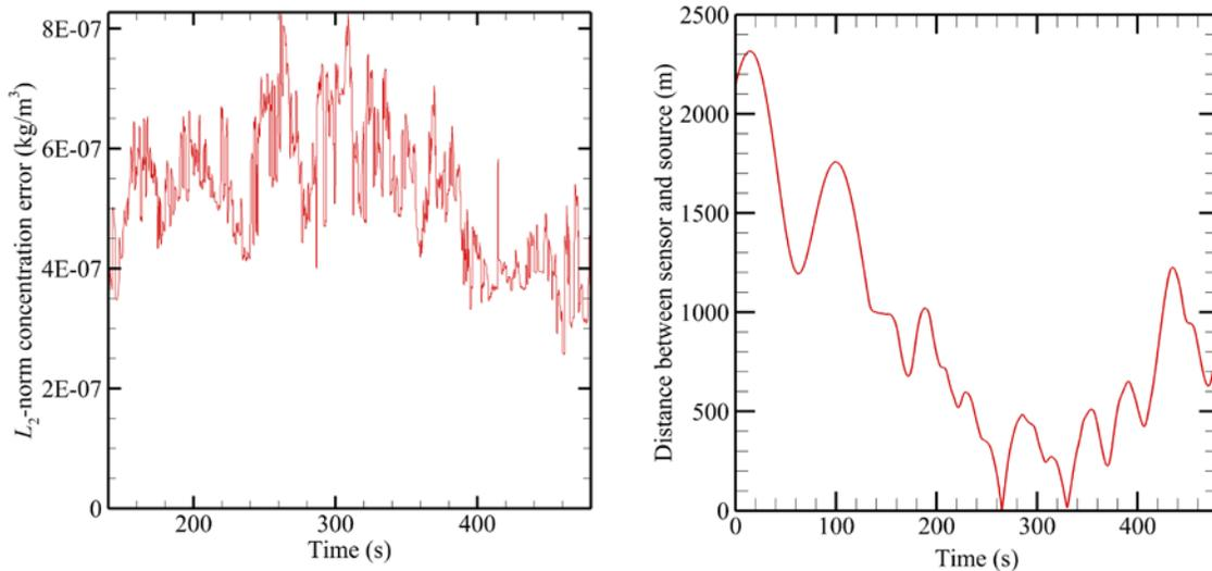
**Figure 28. Estimator performance analysis for a source moving across the domain. (Left) the RMS error vs. time; (right) distance between UAV and source.**
