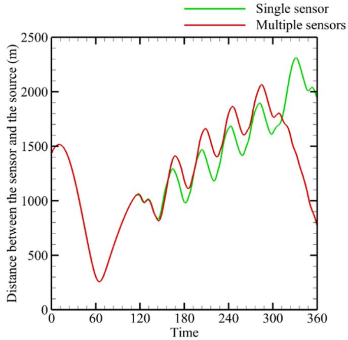
**Figure 36. The distance between the sensor and source versus time for the case of a single sensor and the case of multiple sensors.**
