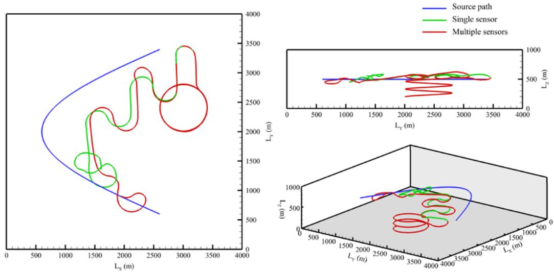
Figure 38. Comparison of the trajectory in case of the concentration estimation with a single sensor and with multiple sensors; the source is moving along an arc trajectory.
