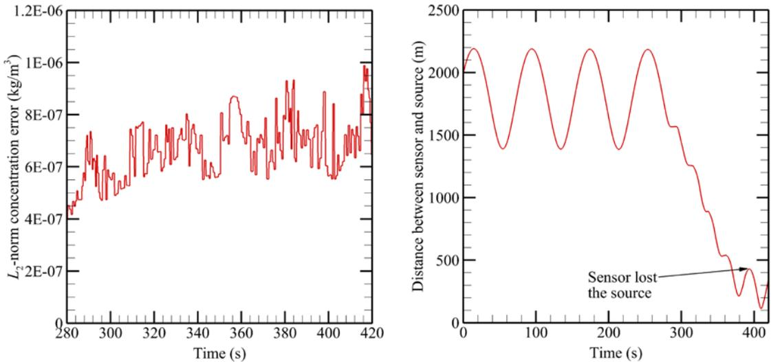
**Figure 22. Estimator performance analysis for a stationary source. (Left) the RMS error vs. time; (right) distance between UAV and source.**
