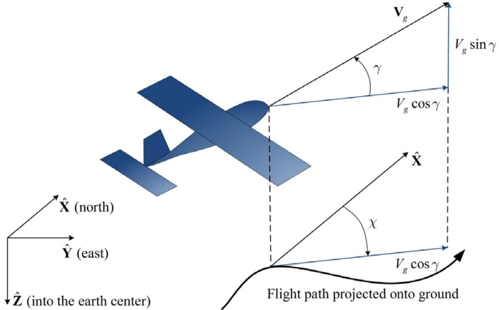
Figure 8. The flight path angle and the course angle.
