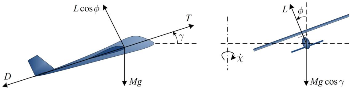
Figure 10. Free-body diagram of the forces acting on the UAV in the climbing coordinated turn.
