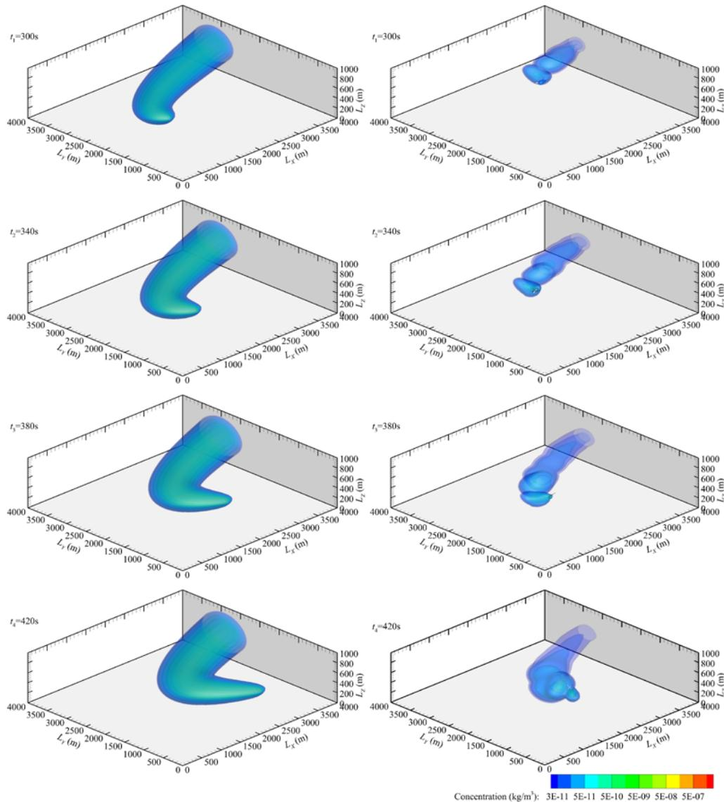
Figure 26. Comparison between estimated plume concentration (left) and simulated concentration (right) for a source moving along an arc trajectory.
