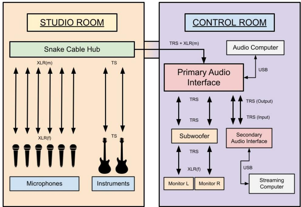
Figure B: Audio Equipment Wiring Guide
