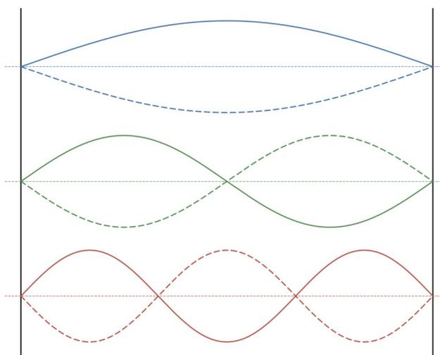
Figure 1.1: First Three One-Dimensional Standing Wave Modes
