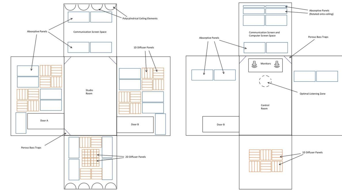
Figure A: Acoustic Designs for Studio and Control Rooms
