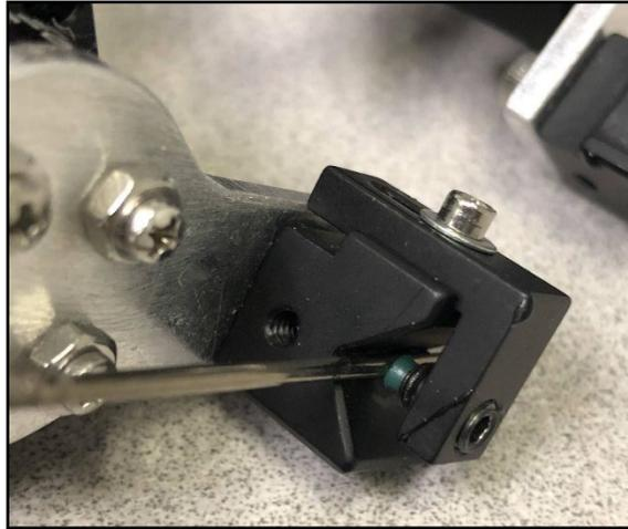
**Figure 2-3: V-groove clamp to hold fiber tube.**
