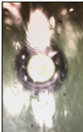
**Figure A-15: Ideal trap should be preserved during the transfer process. The bead is 15.45 micrometers in diameter.**
