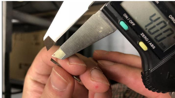
**Figure A-5: 4 mm of fiber extrusion from the tube.**
