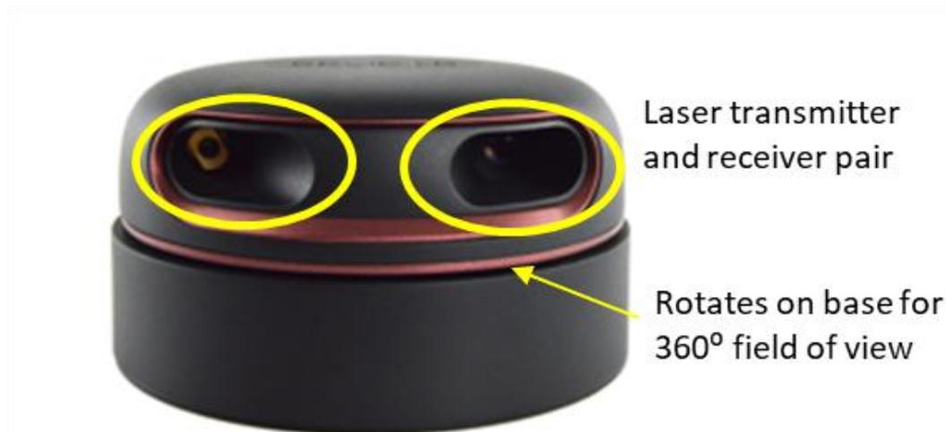
*Figure 13: RPLIDAR A2 LIDAR Sensor. The sensor features a laser transmitter and receiver for determining object distance through reflections. The sensor's housing is able to rotate 360 degrees on the base for maximum field of view. [79]*
