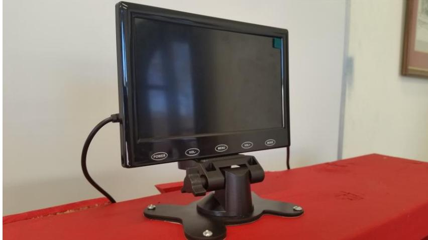
*Figure 39: 800x480 resolution VGA screen that was used to display a visual alarm. Screen turns green (No Danger), yellow (Danger Warning zone) or red (Critical Action zone) based on the location of the object.*
