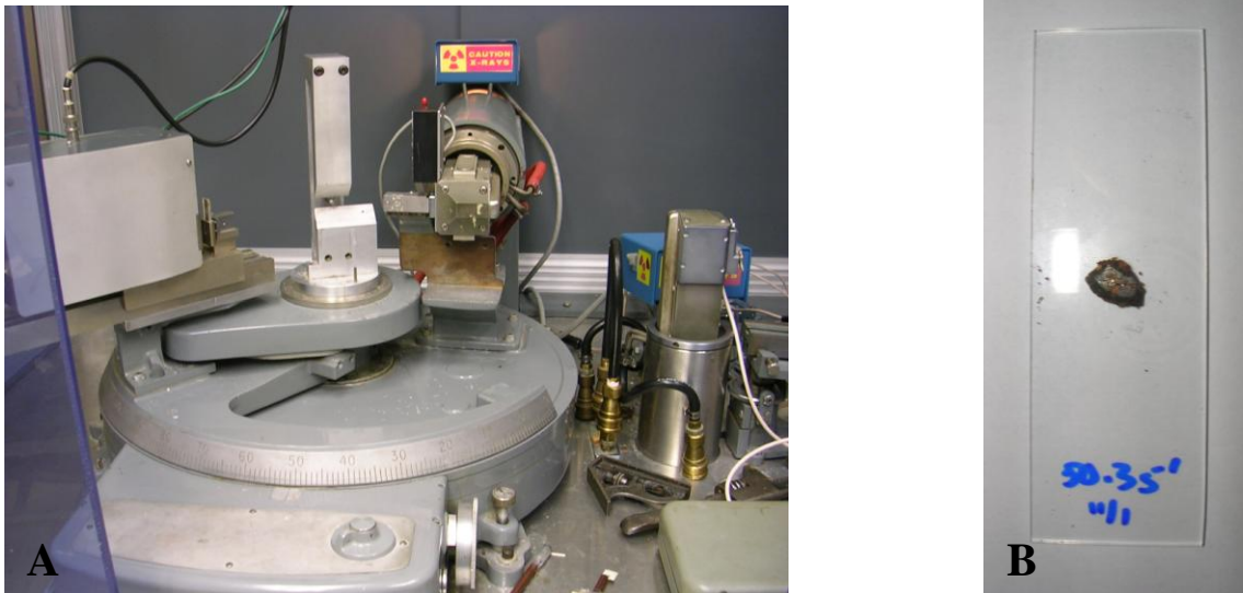
Figure 22: A) Set up for GE/Diano X-Ray Diffractometer B) Example of a prepared sample
