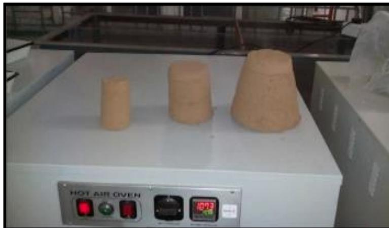
*Figure 6: Different ceramic filter shapes and sizes.*
