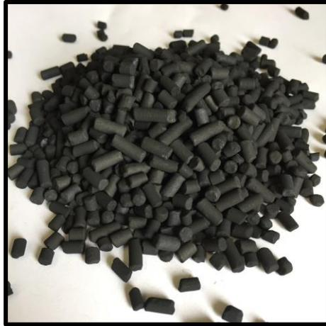
*Figure 3: Activated charcoal pellets.*
