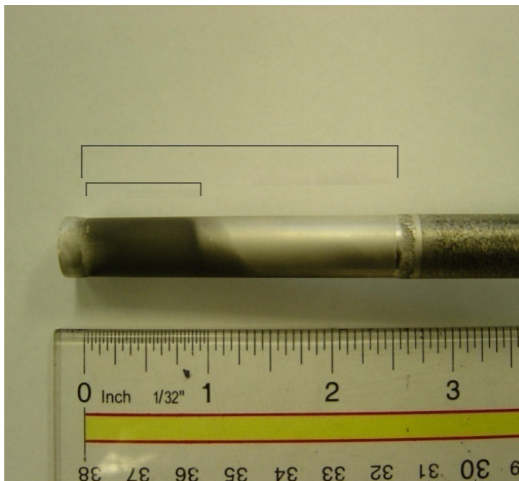
Figure 8.4. Membrane AA-5 appearance after use in WGS experiments.
