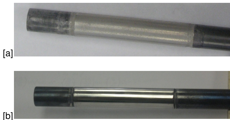
Figure 3.2. Pictures of synthesized membranes [a] Membrane AA-29, unpolished [b] Membrane AA-14, polished and buffed.
