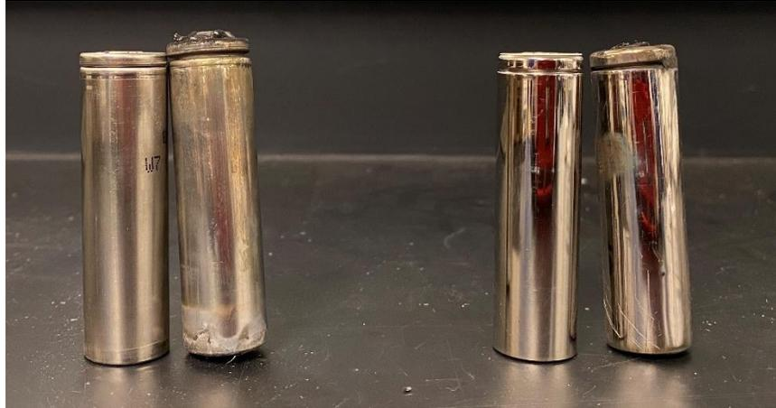
**Figure 2:** Pairs of NMC (left pair) and NCA (right pair) lithium-ion batteries. Within each pair, untested battery cells are on the left and tested battery cells on the right.
