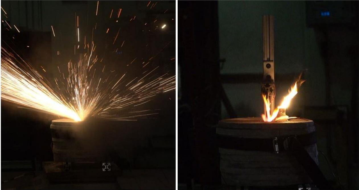
**Figure 7:** Thermal runaway spark streams (left) and flames (right).
