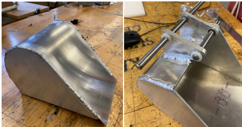
Figure 26: Welding on bucket (before teeth)
