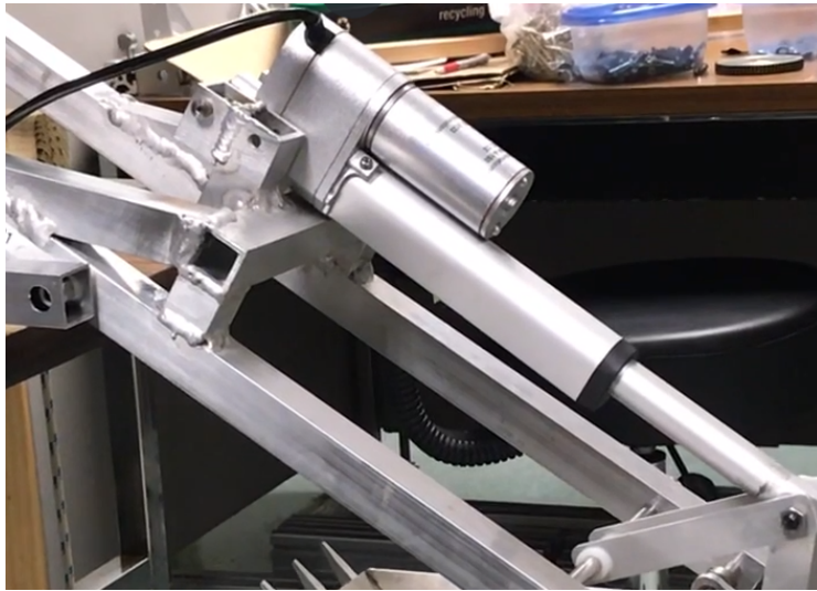
Figure 27: Extended back attachment on linear actuator
