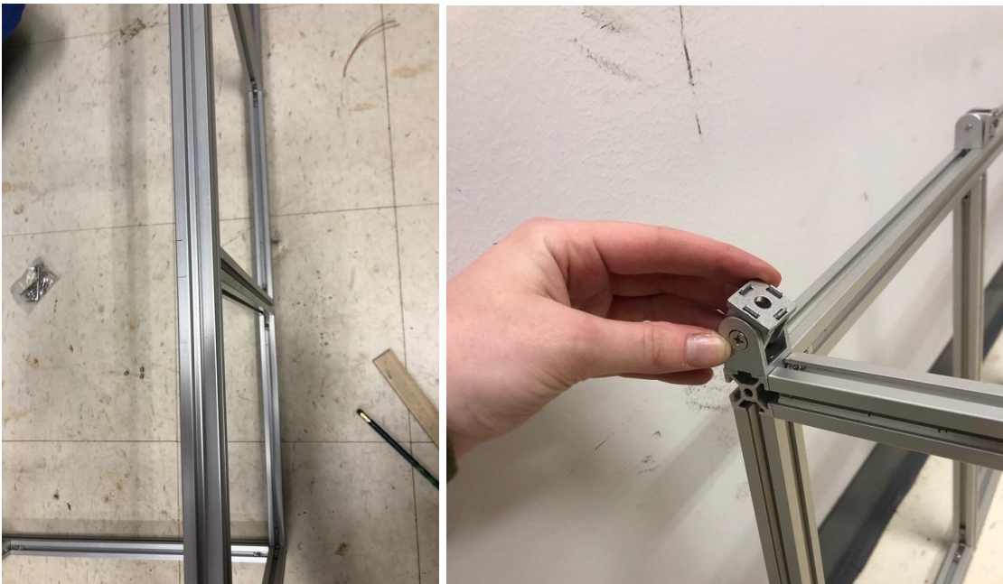
(Image on right shows the correct orientation of the pivot joint on top of the frame)
