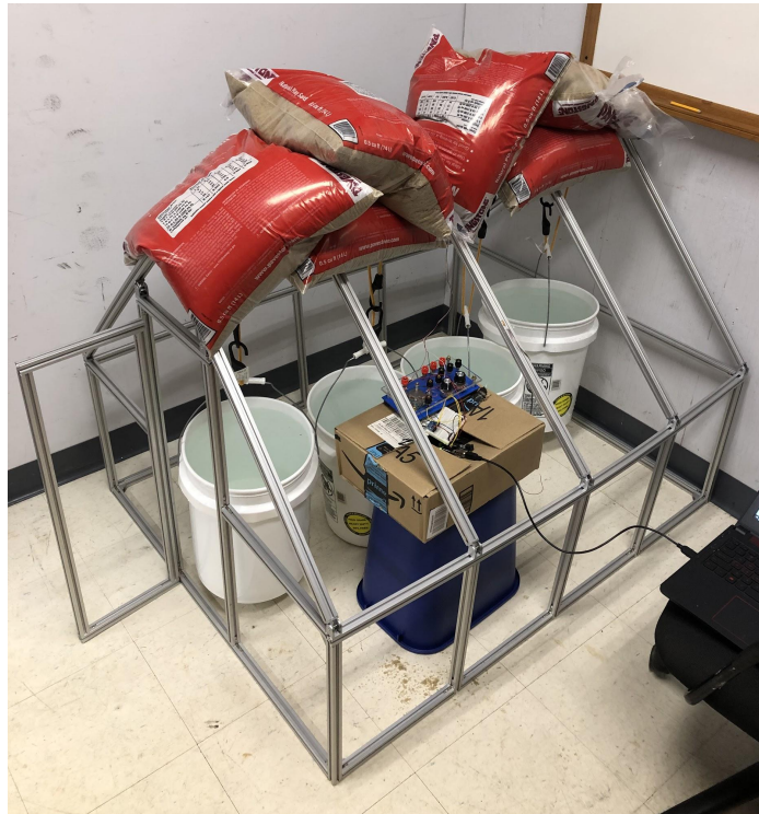
Figure 38: Distributed Load Test on Frame
