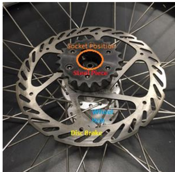
Figure 73: Steel Piece Bolted to Wheel hub and Disc Brake Rotor
