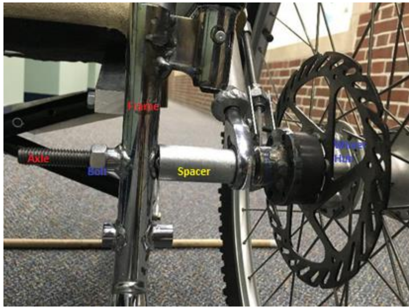
Figure 79: Propulsion System Bolted to Wheelchair Frame
