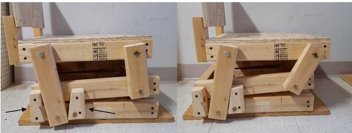
Figure 28: Unequal four-bar linkage. Left: Indoor position. Right: Ideal position for outdoor use. The arrows point to the stops.
