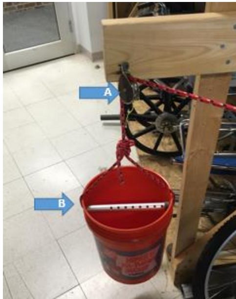
Figure 105: Pulley and Weight Bucket Configuration.
