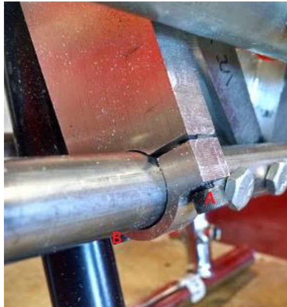
Figure 64: Attachment of the Rectangular link and Clamp to the Frame (Right Side)
