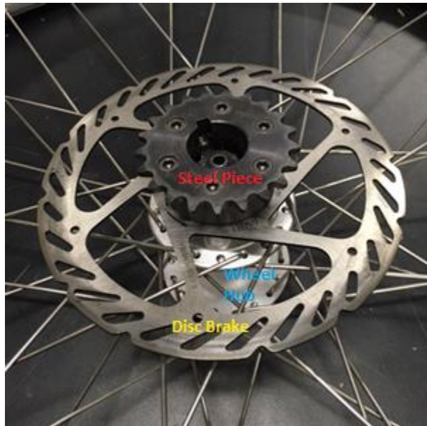
Figure 101: Wheel that was used for Final Prototype.
