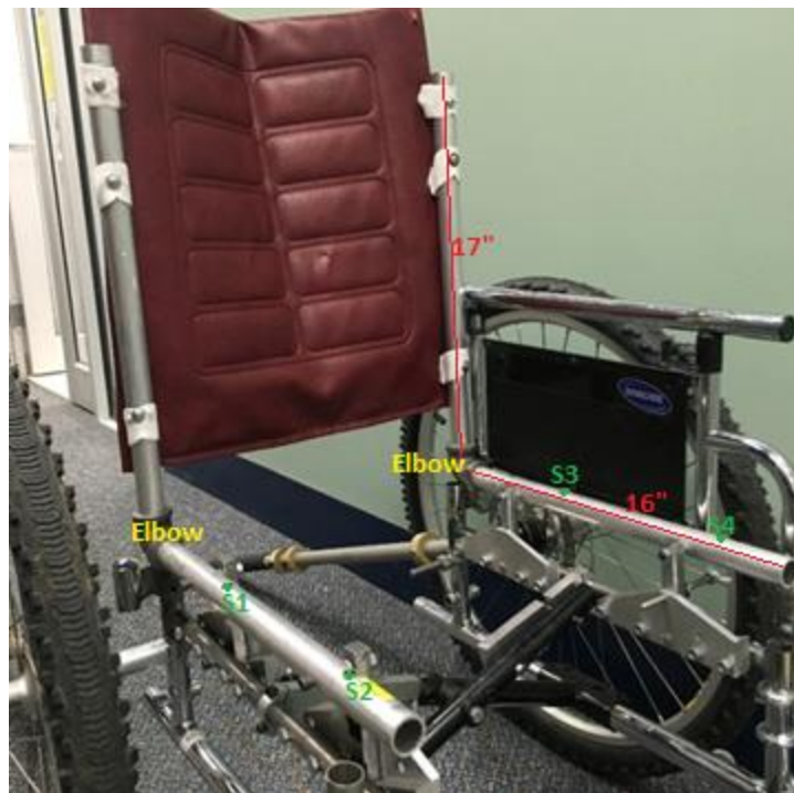
Figure 71: Seat Frame and Seat Back Mounted on Wheelchair
