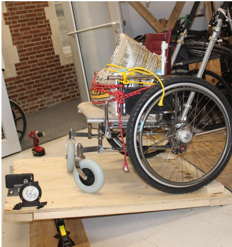
Figure 85: Static Backward Tipping Test Setup
