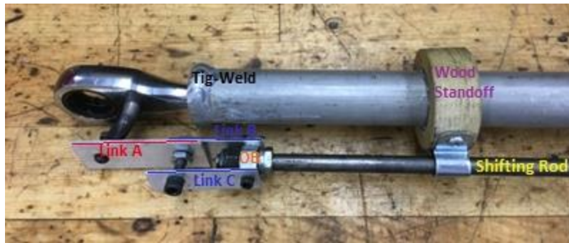
Figure 75: Ratchet and lower end of Drive Lever
