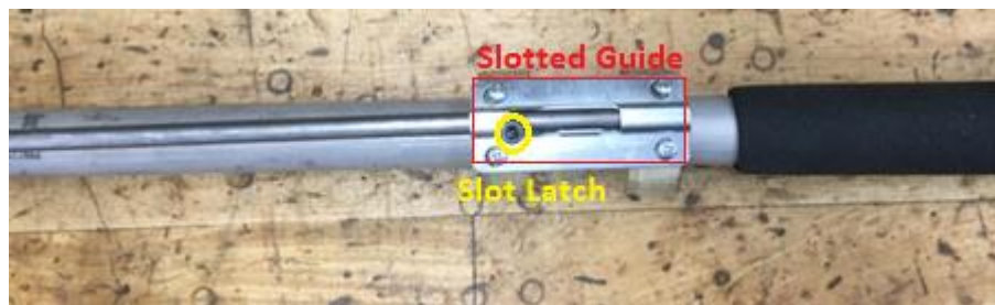
Figure 76: Shifting Mechanism in Forward Position
