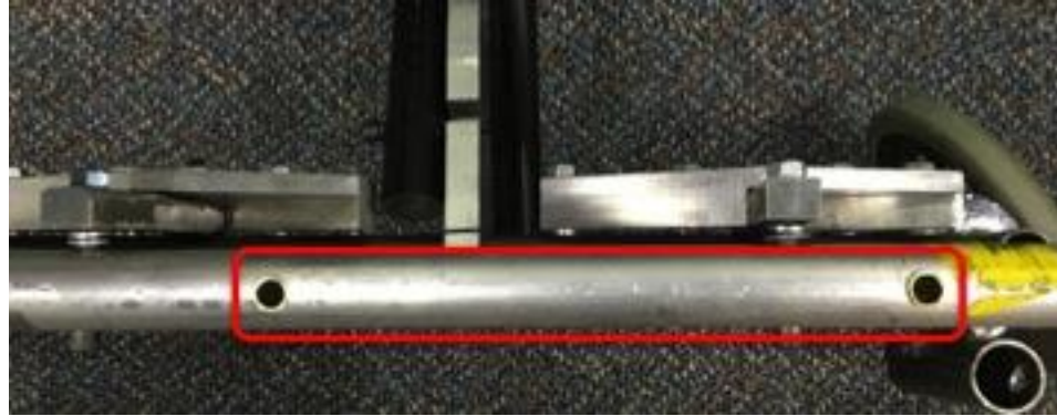
Figure 70: Press Fit Brass Locators on Right Seat Frame (top view)
