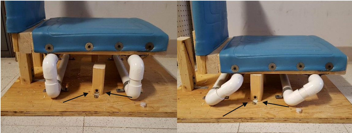
Figure 27: Zero order parallelogram linkage. Left: Indoor resting position. Right: Ideal position for outdoor use. The arrows point to the stops.
