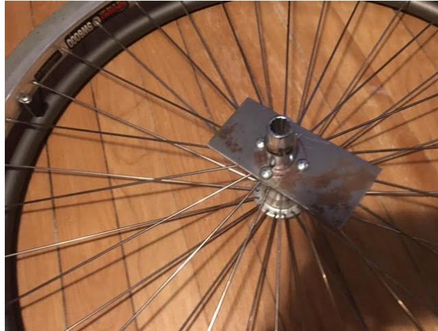
Figure 100: Wheel with Welded Steel Plate and Socket.
