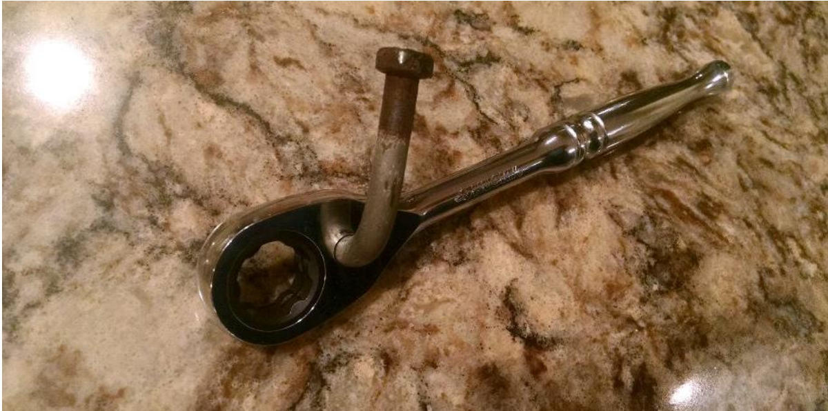
Figure 74: Bent Shifting Rod Inserted into Wrench
