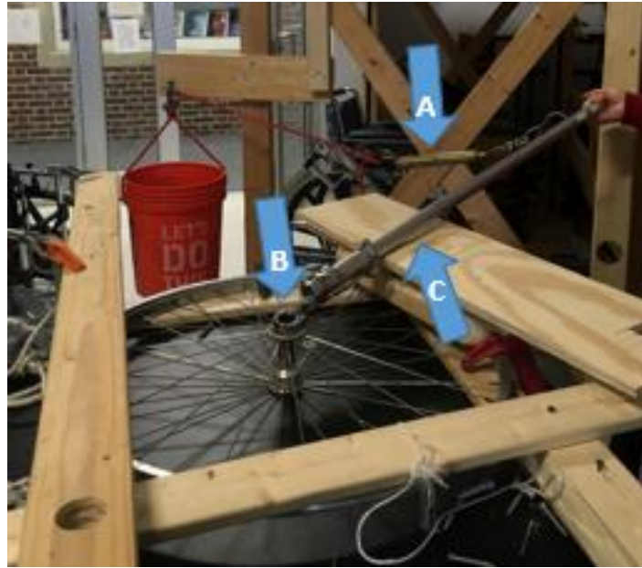
Figure 104: Lever Arm attached to Socket.
