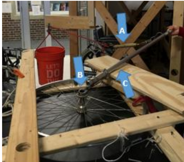
Figure 104: Lever Arm attached to Socket.
