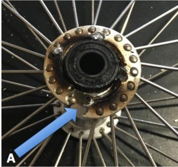
Figure 55: Fracture point of propulsion system (drive lever not pictured).
