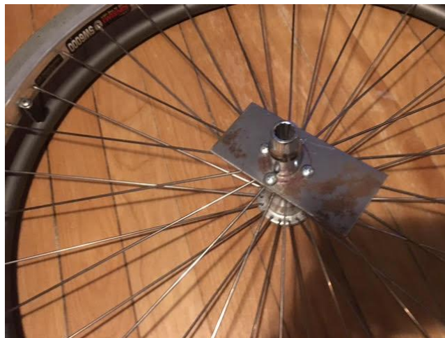
Figure 100: Wheel with Welded Steel Plate and Socket.
