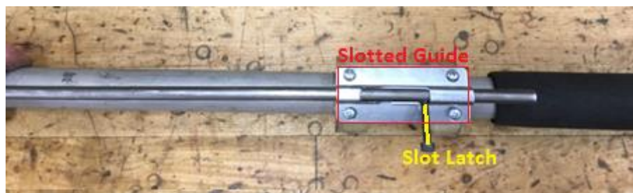
Figure 77: Shifting in Reverse Position
