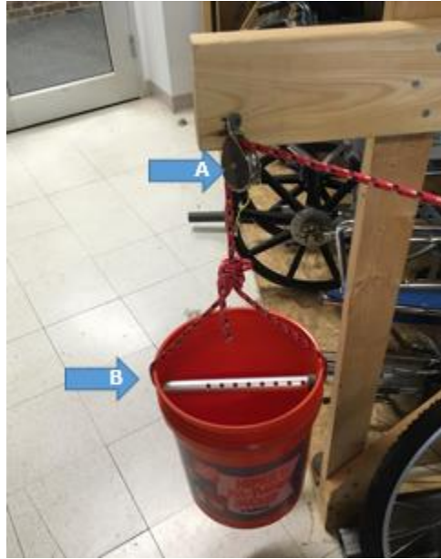
Figure 105: Pulley and Weight Bucket Configuration.
