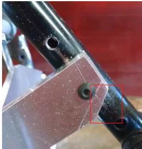
Figure 67: Remedial Cut of Machined Part (Rectangular Link)
