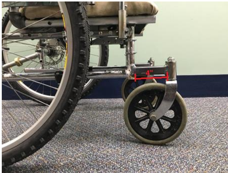
Figure 61: Modified Castor Headset location
