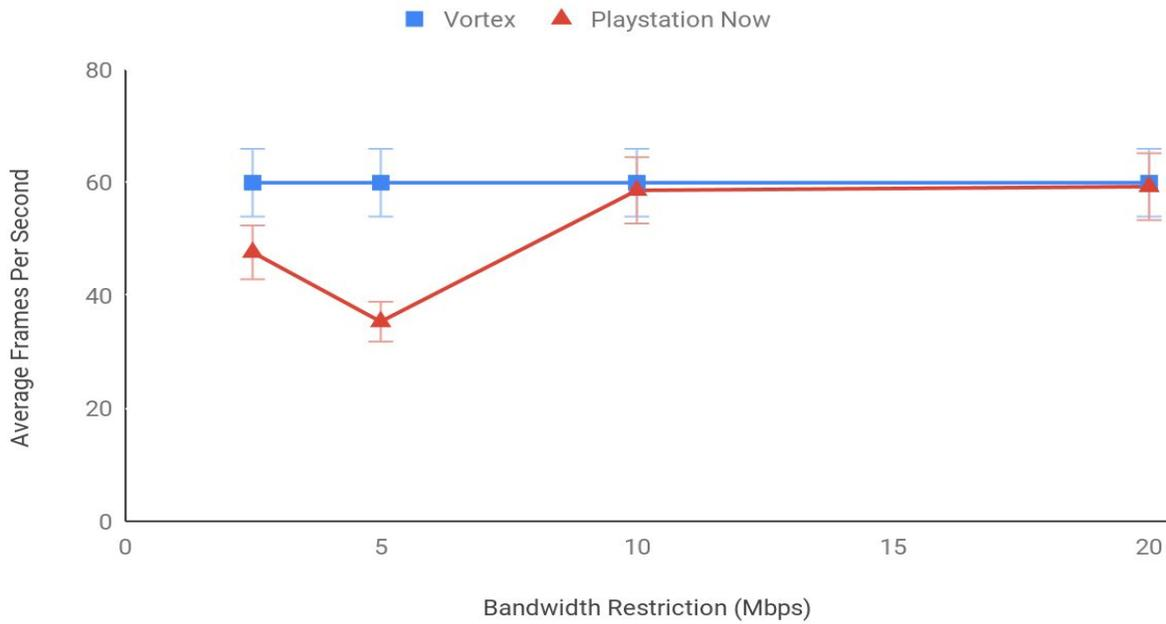
Figure 6: Average Frames Per Second vs. Bandwidth Restriction
