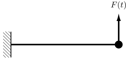
Figure 4.5: SDOF System Subject to Forced Vibration
