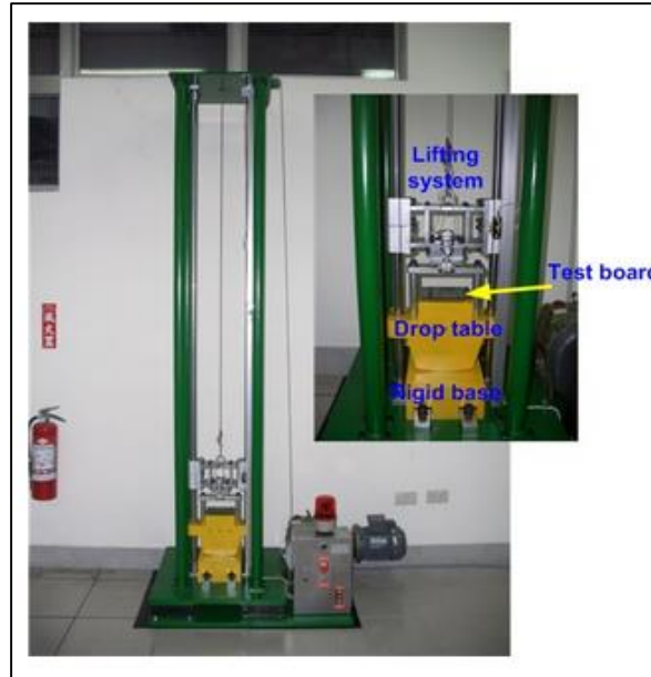
Figure 2-6: Drop Weight Impact Test [65]
