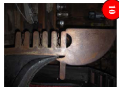
This is the ferro from the gondola da fresco . The ferro is the distinctive metal design at the prow, or front, of the gondola and similar types of boats. The unique shape of the ferro is famous worldwide – popular tradition maintains that the sixteenth century Venetian, the elegant curve signifies the Doge's cap, or the Grand Canal.
