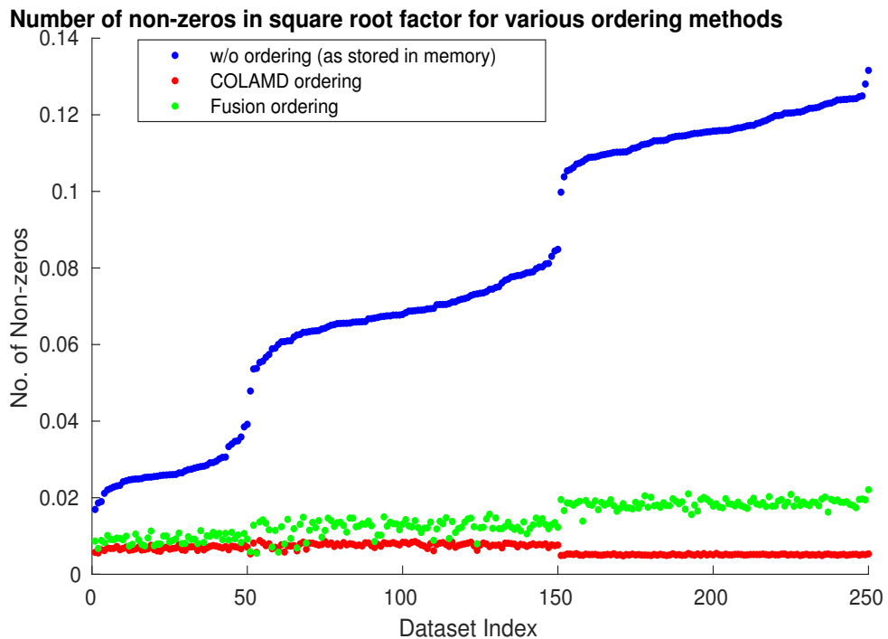
FIGURE 3.7: Comparison among different ordering schemes on the number of non-zero fill-in produced. It can be seen that the COLAMD produces the least and is closely followed by fusion ordering. On the other hand, the variable memory order produces huge fill-in.
