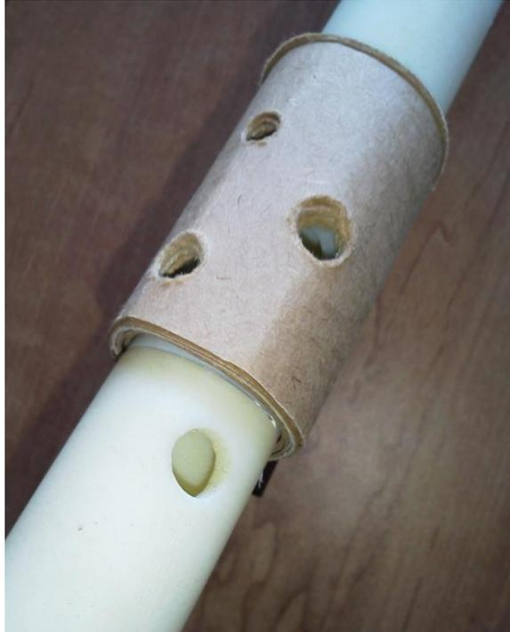
**Figure 25: Set up using Cardboard to Increase Chimney Heights**
