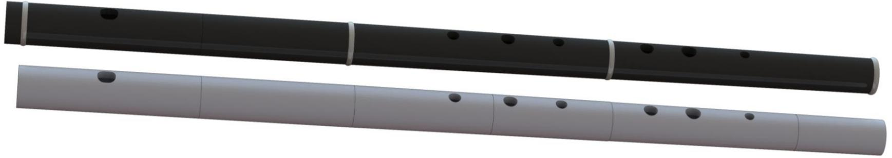
Figure 19: SolidWorks Models of Delrin® (top) and Initial Rapid Prototype (bottom)
