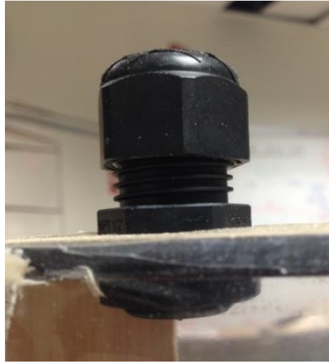
Figure 48: Installed Drainage System
