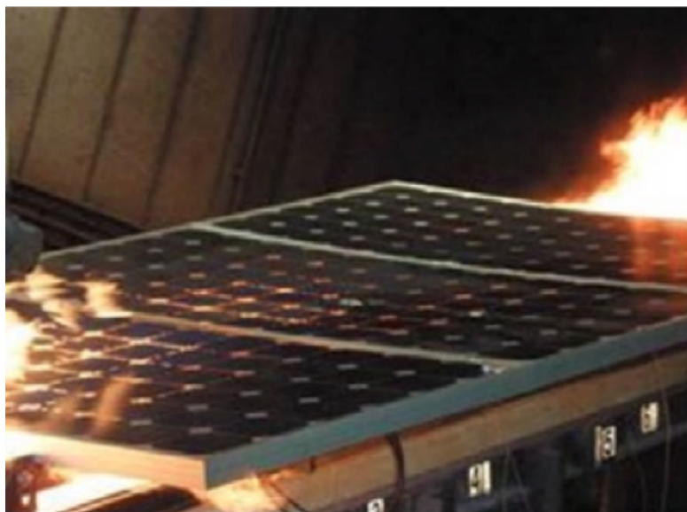
Figure 13: Spread of Fire Test Underneath Solar Panels (Sherwood et al., 2013)
