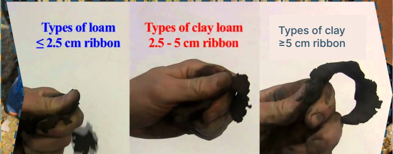
Figure 10: Examples of different soil types during the ribbon test.
